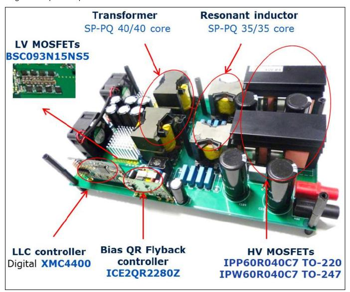
Figure 14 The 3 kW dual-phase LLC demo board
