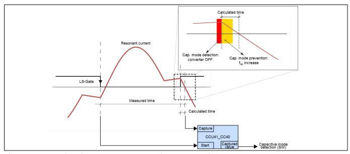
Figure 29 CCU4 timer in capture mode to adquire the phase difference between voltage and current and capacitive mode prevention and detection phase thresholds.
