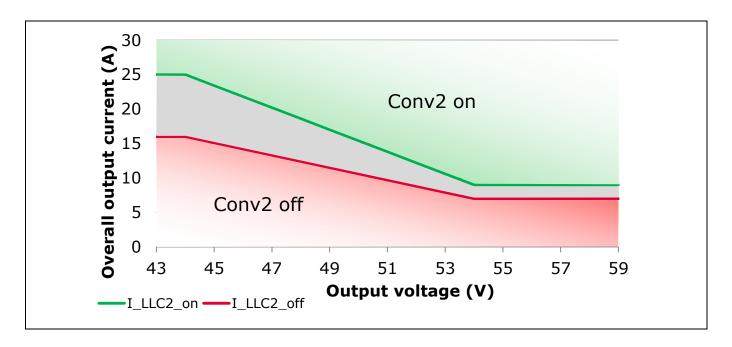
Figure 23 LLC Conv2 shedding depends on overall output current thresholds for a given target voltage.
