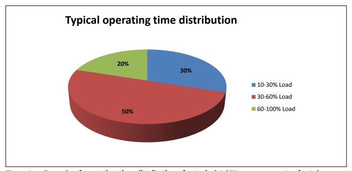
Figure 9 Example of operating time distribution of a typical 3 kW power converter for telecom or industrial application
