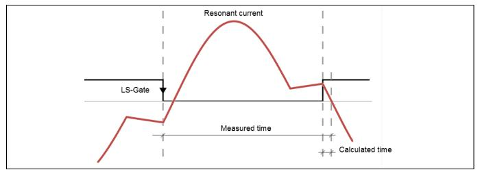
Figure 12 Capacitive load mode prediction & protection concept
