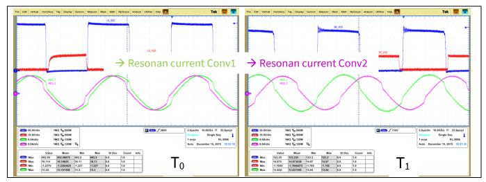
Phase difference of phase 1 (green) and phase 2 (purple) resonant currents at the same power Figure 21 at two different moments in time.
