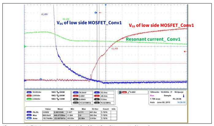
Figure 37 Full ZVS turn-on at only 3% load (90 W) and  $V_{in}$  = 380  $V_{DC}$  (Conv1)
