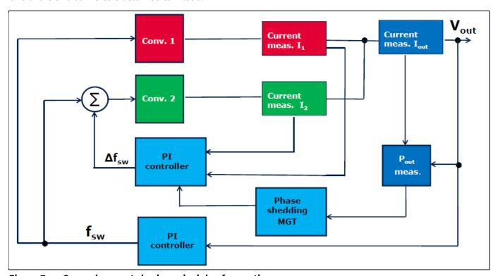
Figure 7 General current sharing principle of operation
