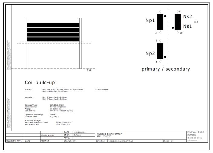
The transformer is produced by Infineon trusted partners in development and manufactuting of magnetic components:
