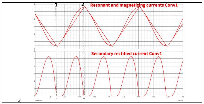
Figure 5 Resonant, magnetizing and seconday rectified currents in case Lr2 is 5% smaller than Lr1
