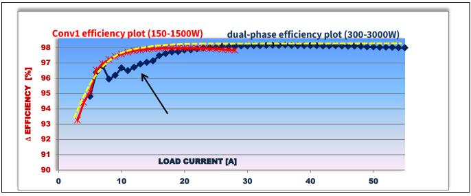
Figure 43 Single versus dual-phase efficency plot comparison
