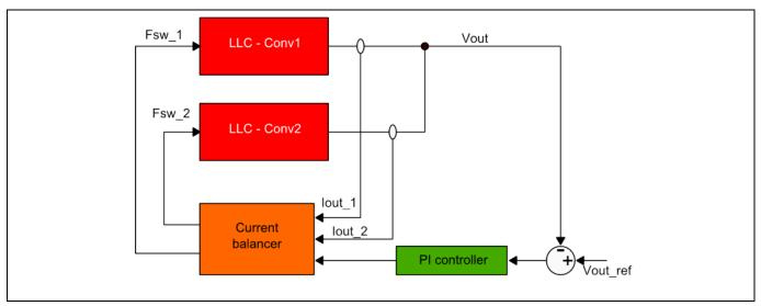
Figure 22 Block diagram of the current sharing and phase shedding functionalities.
