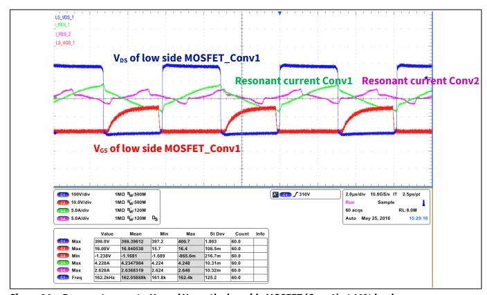
Resonant currents;  $V_{gs}$  and  $V_{ds}$  on the low side MOSFET (Conv1) at 10% load Figure 34
