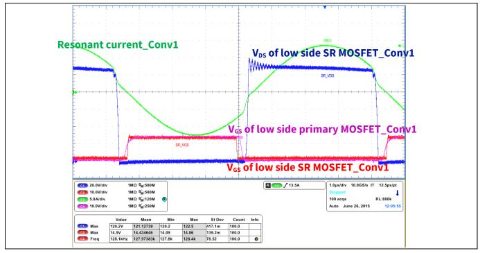
Figure 40 SR MOSFET operation at Full Load and V<sub>in</sub>= 380 V<sub>pc</sub> (Conv1)
