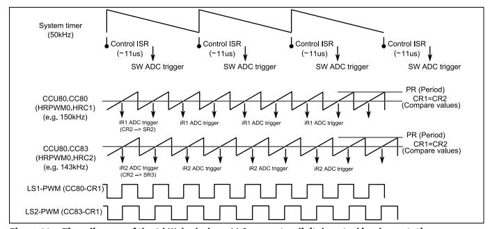
Figure 20 Time diagram of the 3 kW dual-phase LLC converter digital control implementation.
