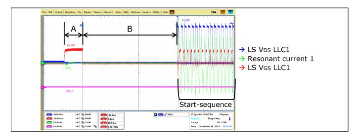
Figure 26 Pre-charge phase scope capture [Ch1=LS\_Vds<sub>1</sub>; Ch2=LS\_Vgs<sub>1</sub>; Ch3=Ires<sub>1</sub>; Ch4=Ires<sub>2</sub>].
