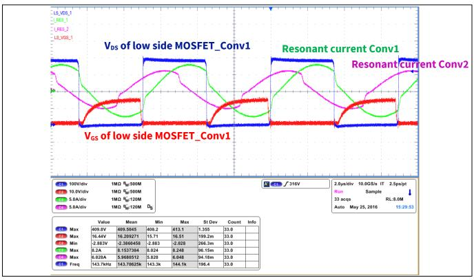
Figure 35 Resonant currents;  $V_{gs}$  and  $V_{ds}$  on the low side MOSFET (Conv1) at 50% load
