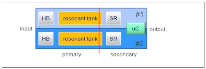
Figure 13 3 kW dual-phase LLC: basic concept
