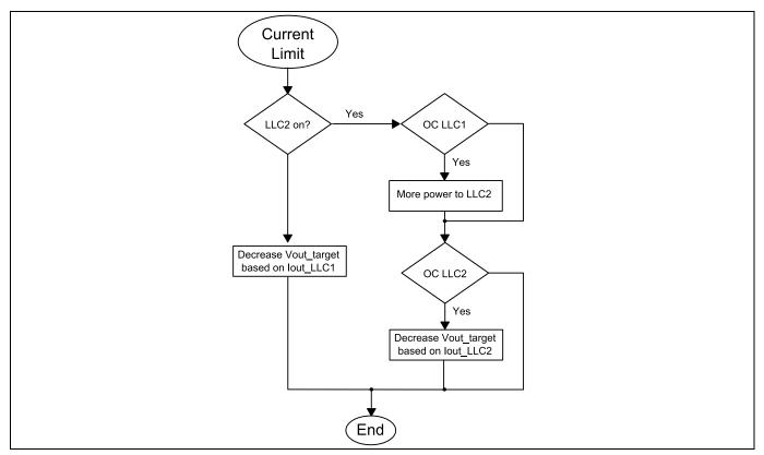
Figure 31 Flow diagram of the current limit algorithm
