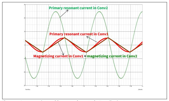
Figure 4 Resonant and magnetizing currents in case Lr2 is 5% smaller than Lr1
