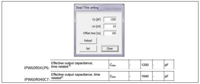
Figure 33 GUI window to provide the necessary parameters for adaptive dead time calculation and C₀ for IPW60R041P6 and IPW60R040C7 CoolMOS™ transistors extracted from the datasheet
