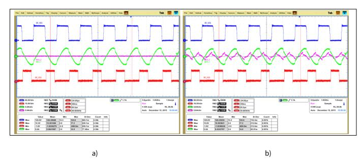
Figure 24 Resonant current of phase 2 (purple) for single phase operation (a) and when phase 2 is enabled (b) after the current threshold is reached.
