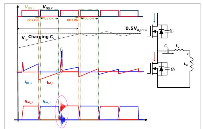
Figure 11 Hard commutation during HB LLC start-up sequence
