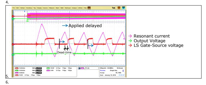
Figure 27 LS-HS driving signal change is applied with a delay after the resonant current crosses zero to guarrante current polarity change and avoid hard-conmutation.
