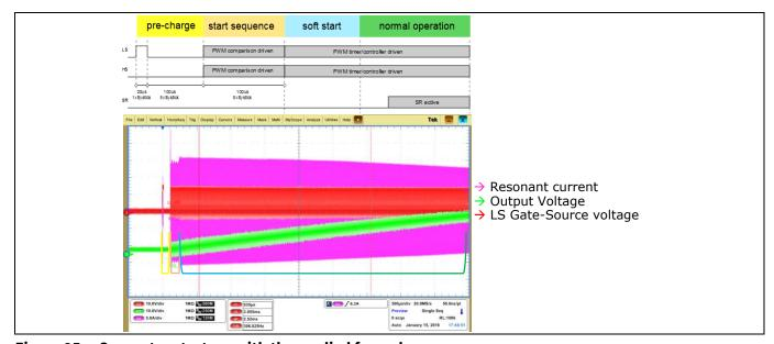
Figure 25 Converter start-up with the applied four-phase sequence.
