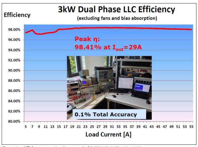
Figure 41 Efficiency versus Load measured with IPW60R040C7 at V<sub>in</sub>=380V<sub>DC</sub>
