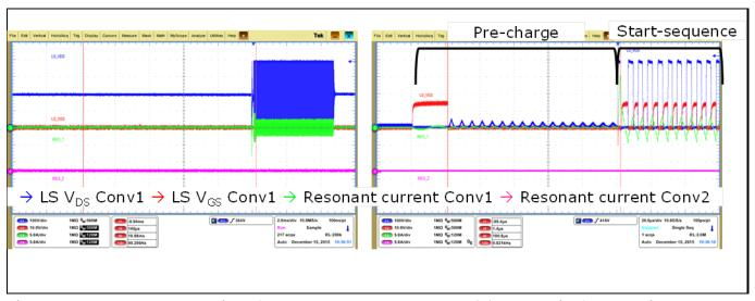
Figure 32 Burst mode operation of the dual-phase LLC converter (a) and detail of the starting sequence during burst mode (b)
