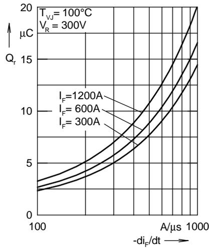
Fig. 2 Typ. reverse recovery charge  $Q_r$  versus  $-di_F/dt$
