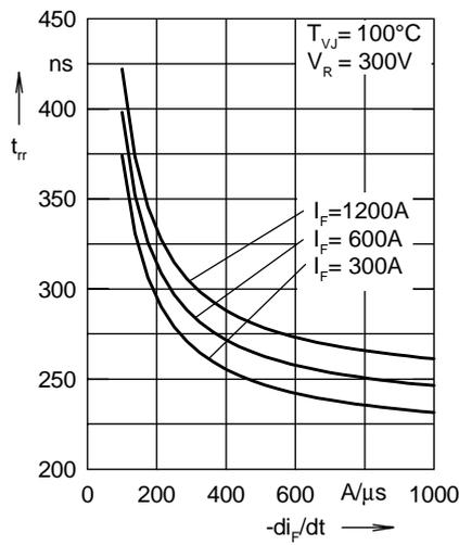
Fig. 5 Typ. recovery time  $t_{tr}$  versus  $-di_F/dt$
