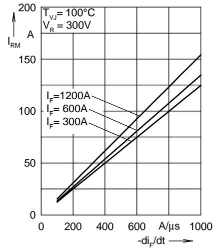
Fig. 3 Typ. peak reverse current  $I_{RM}$  versus  $-di_F/dt$
