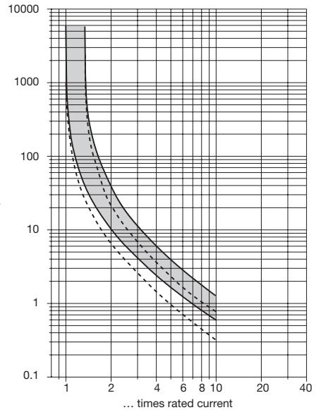
The time/current characteristic curve depends on the ambient temperature prevailing. In order to eliminate nuisance tripping, please multiply the circuit breaker current ratings by the derating factor shown below. See also section Technical information.
