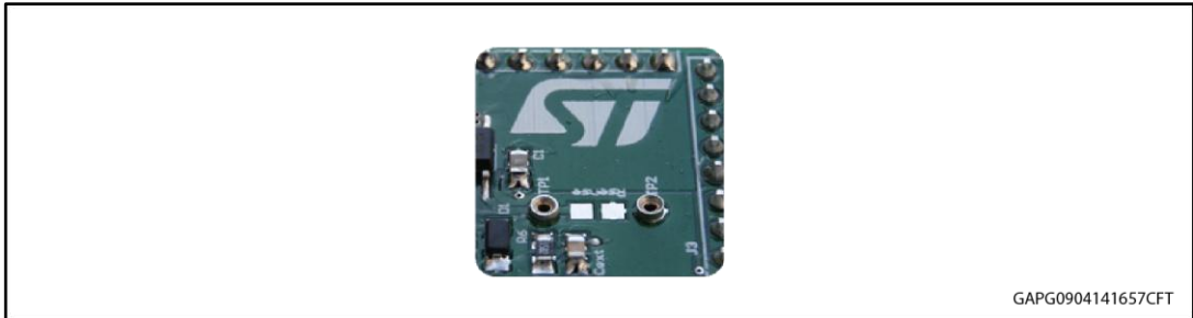
Figure 4: Mounting through-hole sense resistor
