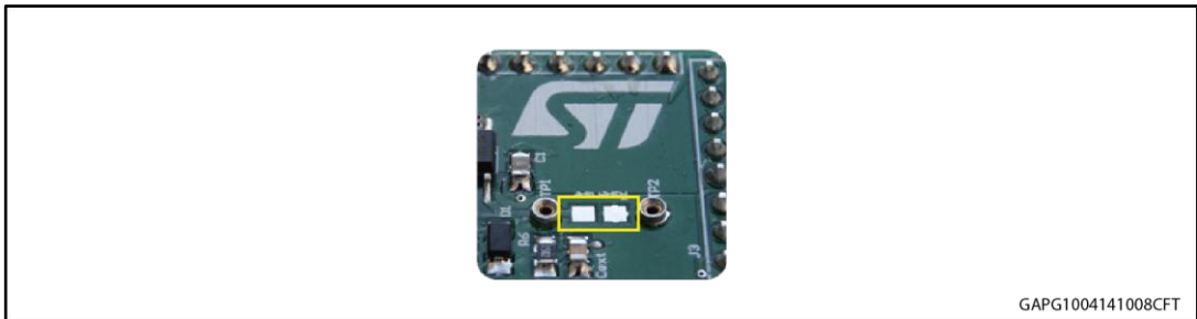
Figure 5: Pads for soldering SMD resistor
