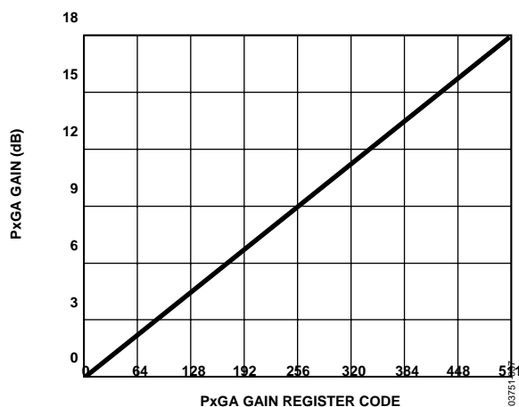
Figure 36. PxGA Gain Curve
