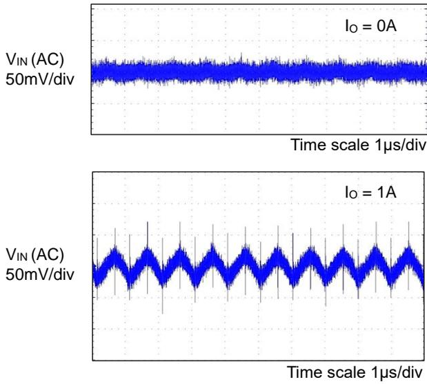
Figure 15. Input Voltage Ripple Wave
