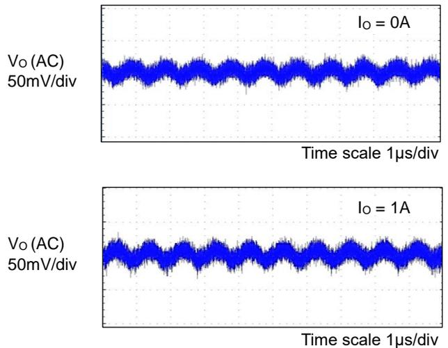
Figure 18. Output Voltage Ripple Wave
