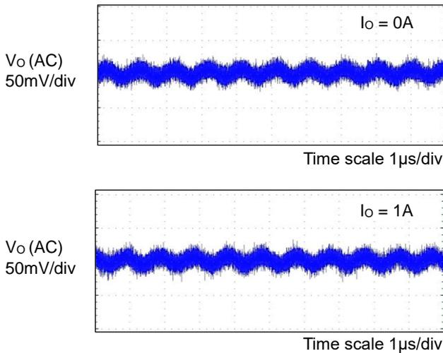
Figure 17. Output Voltage Ripple Wave
