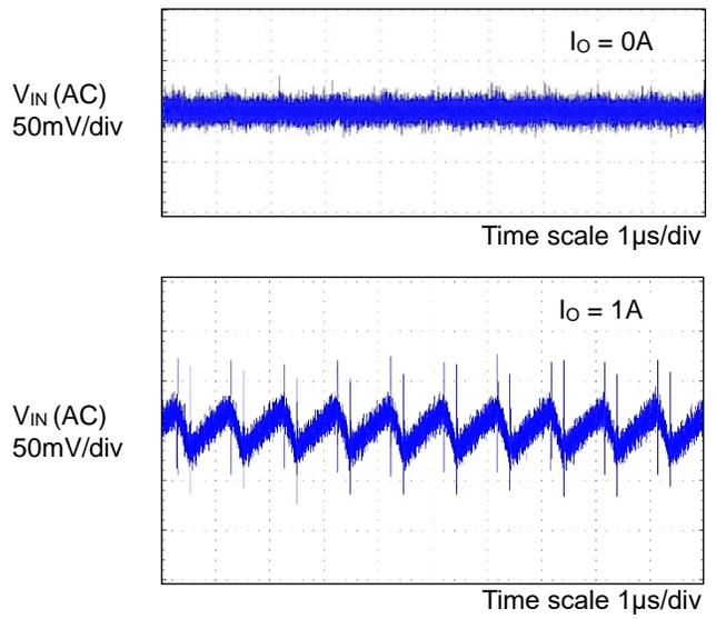
Figure 16. Input Voltage Ripple Wave
