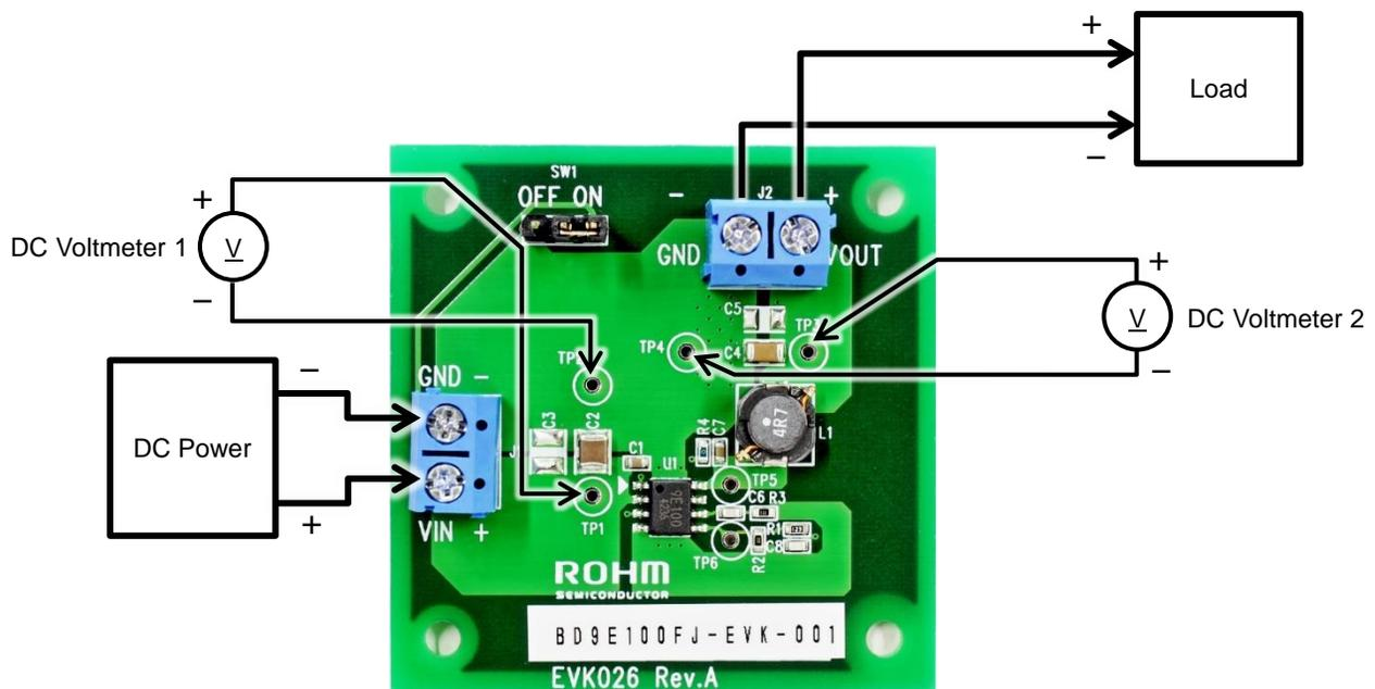
Figure 1. Connection Diagram
