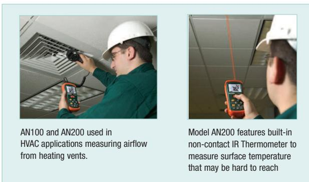
AN100 and AN200 used in HVAC applications measuring airflow from heating vents.
