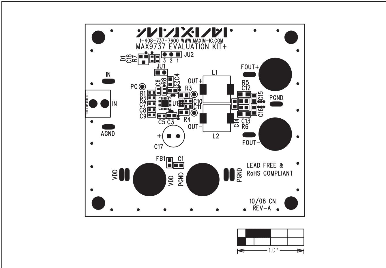
Figure 2. MAX9737 EV Kit Component Placement Guide—Component Side
