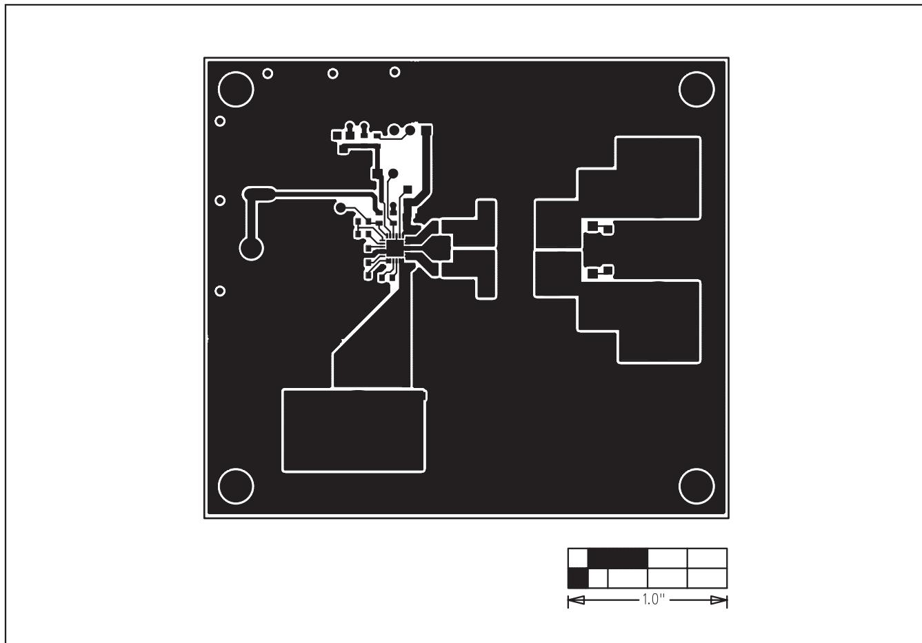
Figure 3. MAX9737 EV Kit PCB Layout—Component Side
