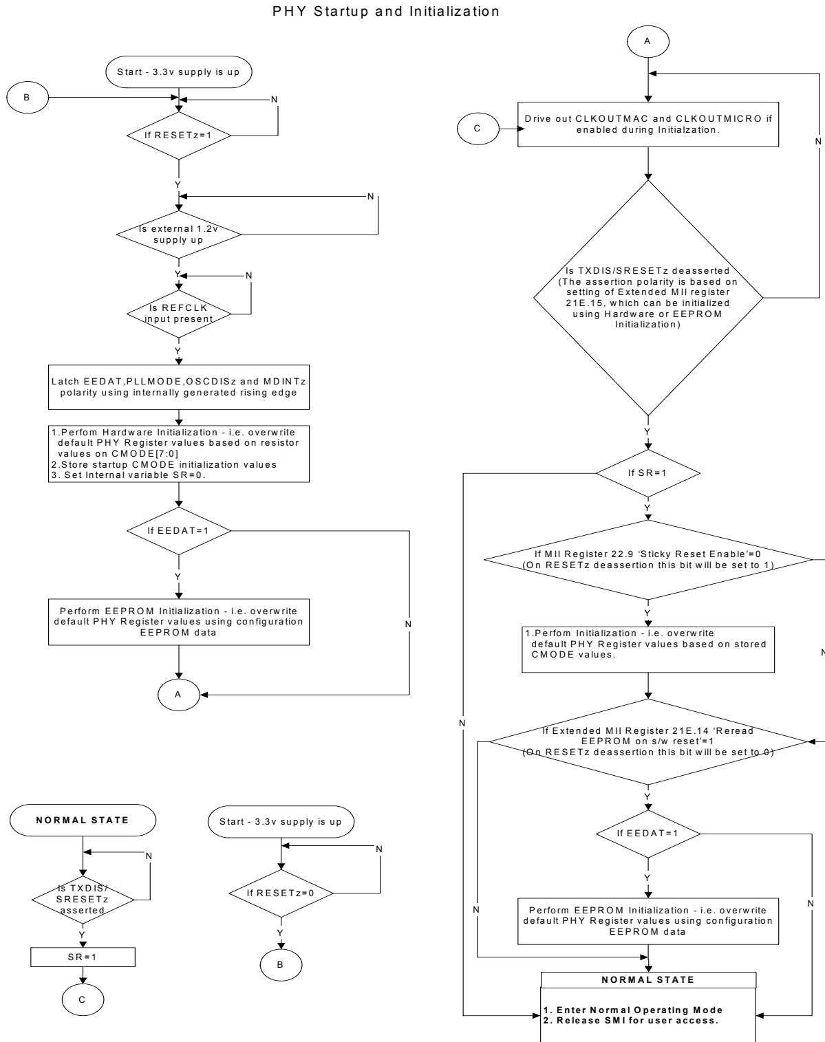
Figure 35. PHY Startup and Initialization Sequence
