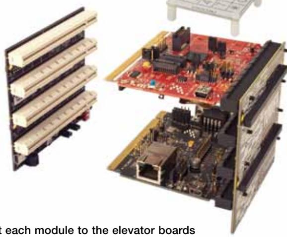
3. Connect each module to the elevator boards
