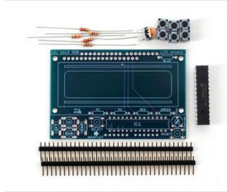
Check the kit against the parts list (https://adafru.it/cl9) to verify you have all the parts necessary
