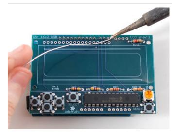
Solder all of the header pins. Even though they aren't used for passing signals, they will make the mechanical connection to the Arduino strong.
