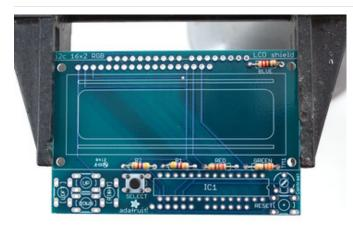
Next up we will place the buttons. These buttons are useful to send a signal to the Arduino (say if you have a basic menu system). We have a 4-way 'direction pad' for up/down/left/right input and a button to the right called SELECT. These 5 buttons should be able to make 'talking' back to your project easy. These are connected to the I2C port expander chip so they require no extra pins on the Arduino, our library does the work of reading whether they are pressed.
