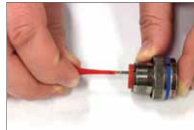
Plastic tool with contact in proper position.
