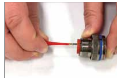
Plastic tool with contact in proper position.
