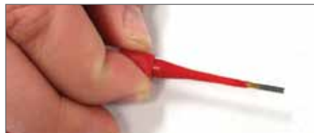
Plastic tool with contact in proper position.
