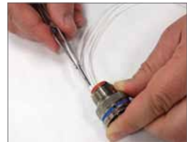
Removal of contacts with metal tool.
