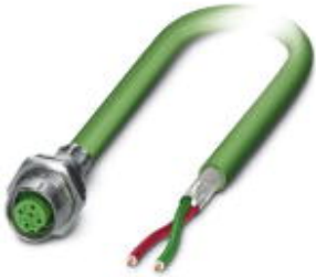
Bus system flush-type socket, PROFIBUS, 2-pos., M12, shielded, B-coded, rear/screw mounting with M16 thread, with 2 m bus cable, 1 x 2 x 0.2 mm 2
