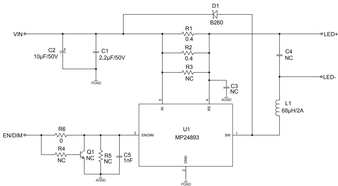
Figure 4: Drive 3 LEDs in Series, 1A Current Output
