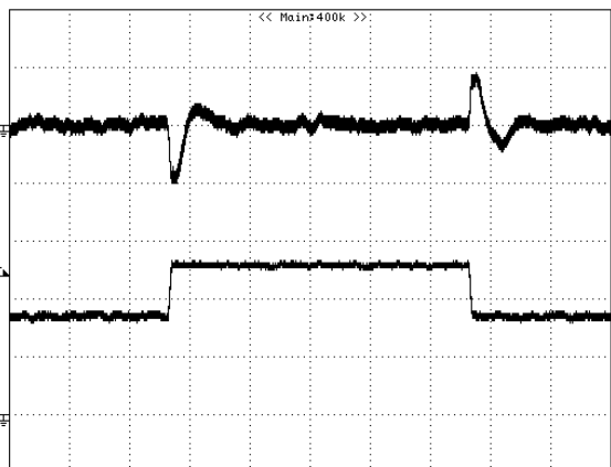
Figure 9: Output voltage response to step-change in load current (75%-50%-75% of I_{o, max} ; di/dt = 1.0A/\mu s ). Load cap: 2000\mu F tantalum capacitor and 1\mu F ceramic capacitor. Top Trace: V_{out} (50mV/div, 200us/div), Bottom Trace: I_{out} (10A/div). Scope measurement should be made using a BNC cable (length shorter than 20 inches). Position the load between 51 mm to 76 mm (2 inches to 3 inches) from the module
