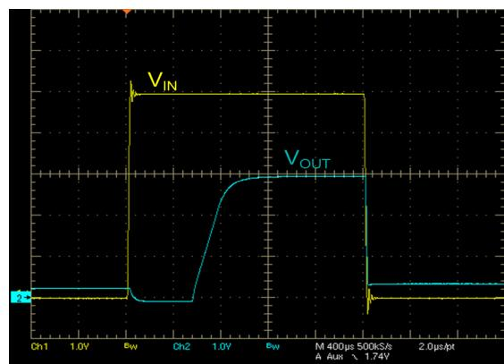
**Figure 13. Startup transient ( $I_{OUT} = 5\text{ mA}$ )**
