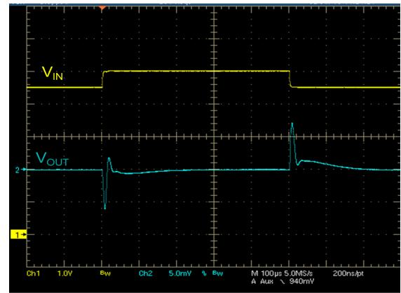
$V_{IN} = 5V$ ,  $V_{OUT}=3V$ ,  $I_{OUT}=1mA$ ,  $C_{OUT}=1\mu F$ ,  $\Delta V_{IN} = 500mV$
