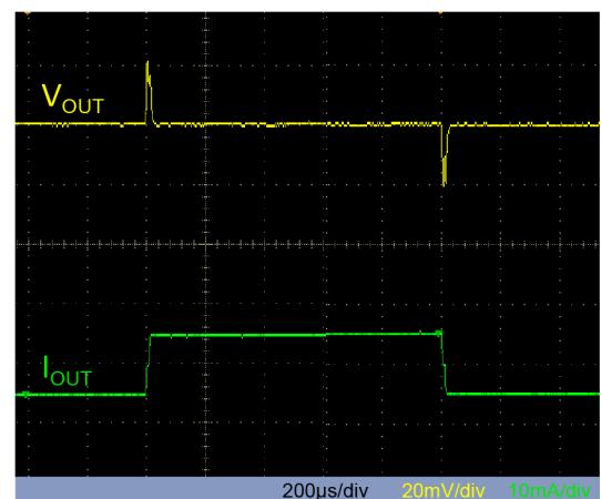
$V_{OUT}=3V$ ,  $I_{OUT}= \pm 5mA$ ,  $C_{IN}=C_{OUT}=1\mu F$
