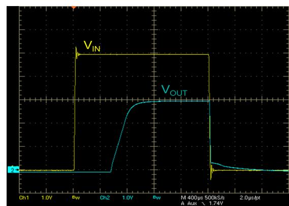
**Figure 14. Line transient (no load)**
