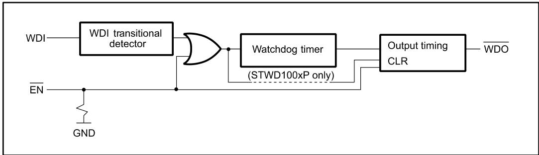
1. If the positive pulse on the enable pin,  $\overline{\text{EN}}$ , is longer than 1  $\mu\text{s}$ , it resets the watch.
