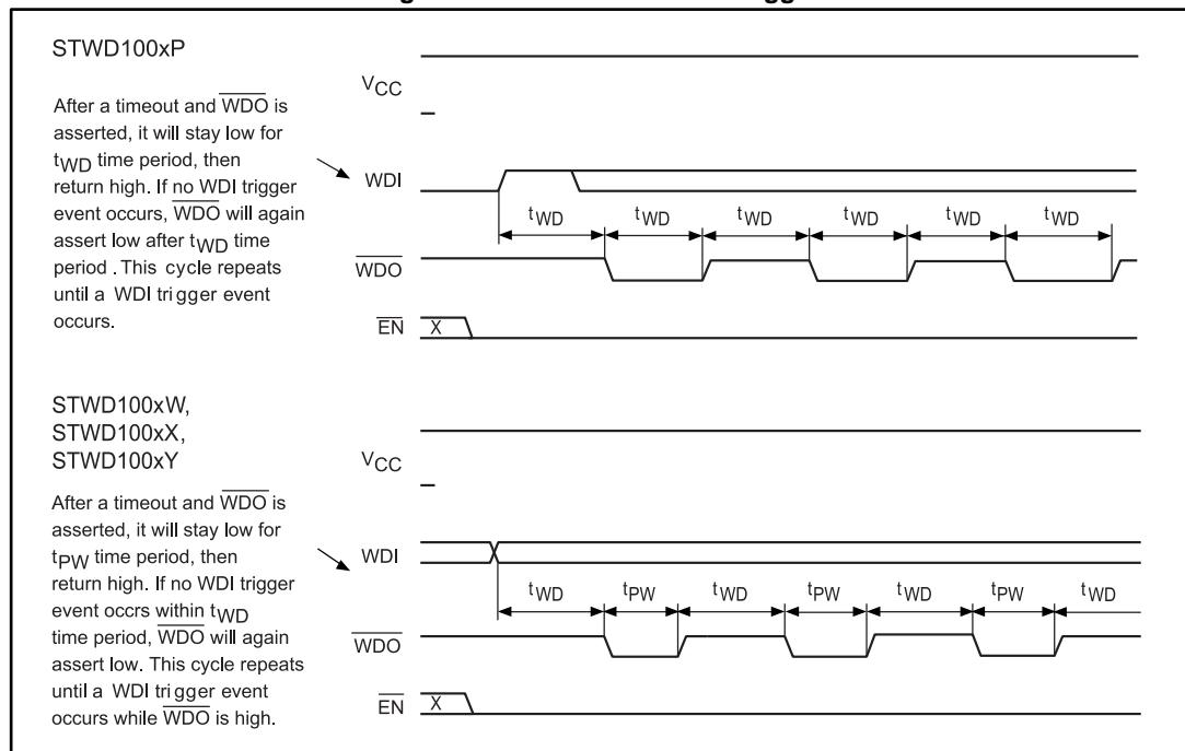
Figure 9: Trigger after timeout
