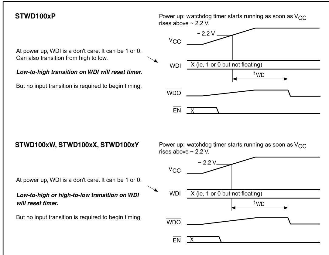
Figure 7: Normal triggering
