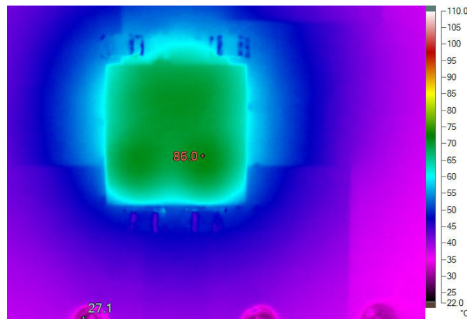
Figure 8. Thermal Capture at 12V IN , 3.3V OUT1 at 18A and 5V OUT2 at 18A (T A = 25°C, 400LFM Airflow and No Heat Sink)
