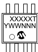
8-Lead MSOP (150 mil)
