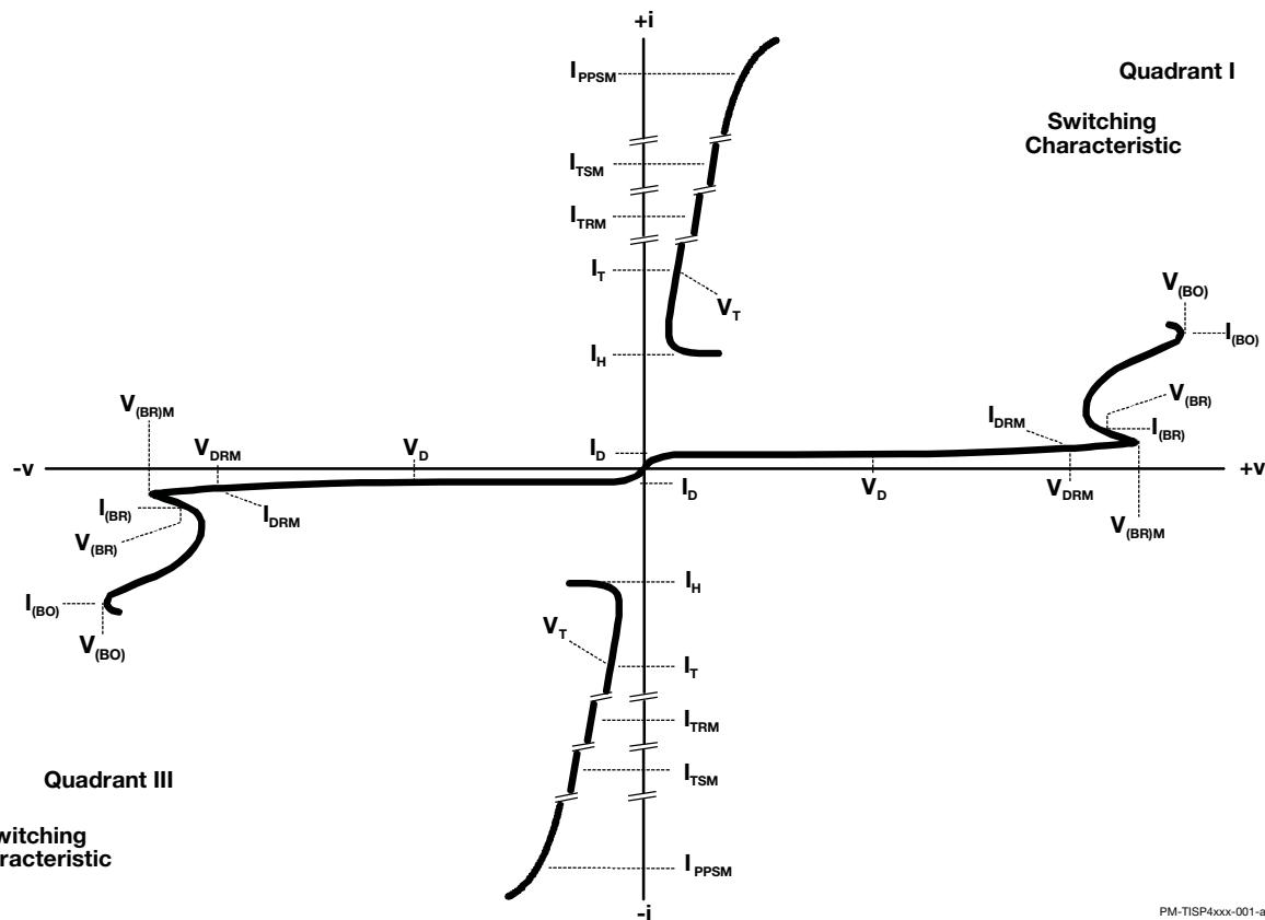
**Figure 1. Voltage-Current Characteristic for T and R Terminals**
