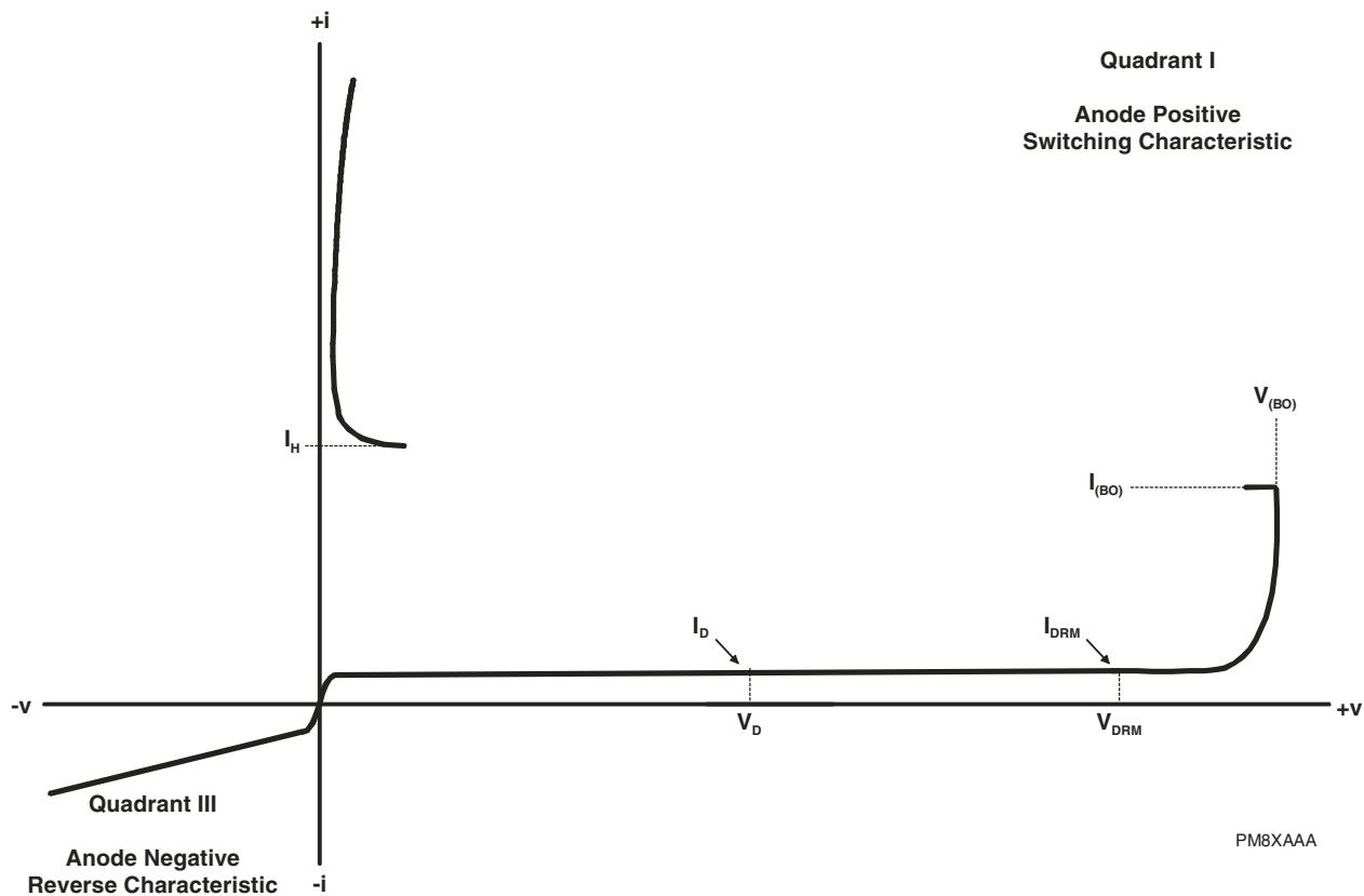
Figure 1. Voltage-Current Characteristic for A and K Terminals
