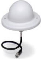
Omnidirectional antenna with protection against vandalism, 2.4 GHz, 3 dBi gain, IP55 degree of protection, 1.5 m cable length, RSMA connection (male), h/v 360°/85° apex angle.
