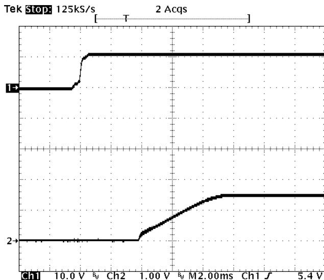
**Fig-1.5V-4:** Turn-on transient for  $V_{out}=1.5V$  with application of  $V_{in}$  at full rated load current (resistive) and  $47\mu F \times 4$  external capacitance at  $V_{in}=12V$ .
