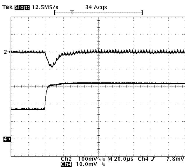
**Fig-1.2V-6:** Output voltage response for  $V_{out}=1.2V$  to positive load current step change from 8A to 16A with slew rate of  $5A/\mu s$  at  $V_{in}=12V$ .  $C_o=47\mu F \times 4$  ceramic.
