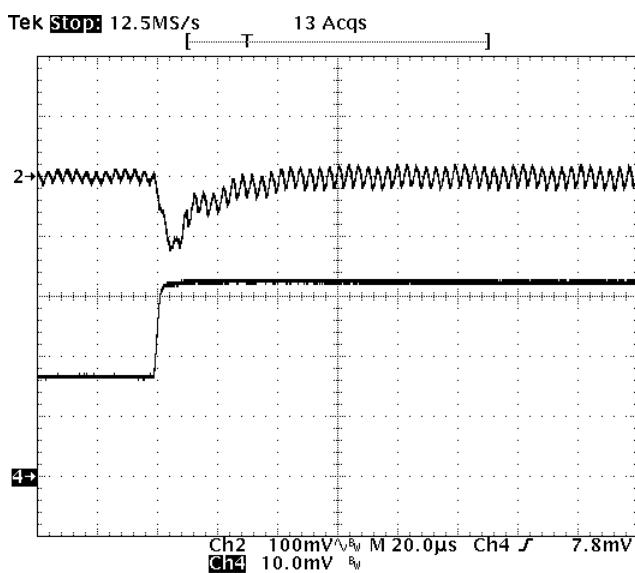
**Fig-5.0V-6:** Output voltage response for  $V_{out}=5.0V$  to positive load current step change from 8A to 16A with slew rate of  $5A/\mu s$  at  $V_{in}=12V$ .  $C_o=47\mu F \times 4$  ceramic.
