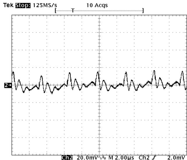
**Fig-1.2V-5:** Output voltage ripple (20mV/div.) for  $V_{out}=1.2V$  at full rated load current into a resistive load with external capacitance  $47\mu F \times 4$  ceramic +  $1\mu F$  ceramic at  $V_{in}=12V$ .
