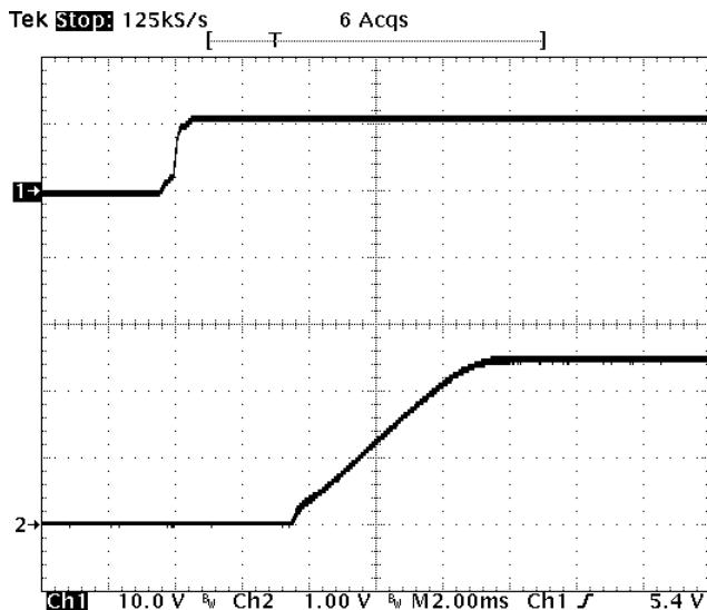
**Fig-2.5V-4:** Turn-on transient for  $V_{out}=2.5V$  with application of  $V_{in}$  at full rated load current (resistive) and  $47\mu F \times 4$  external capacitance at  $V_{in}=12V$ .
