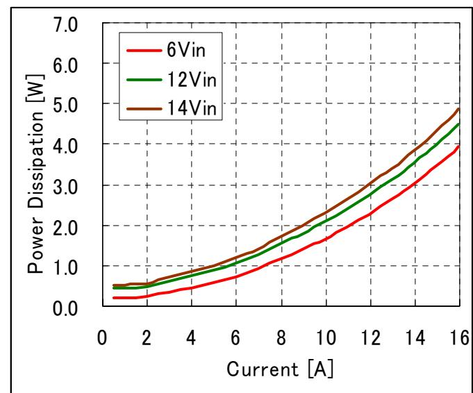
**Fig-2.0V-3:** Power Loss vs. load current and input voltage for  $V_{out}=2.0V$ .
