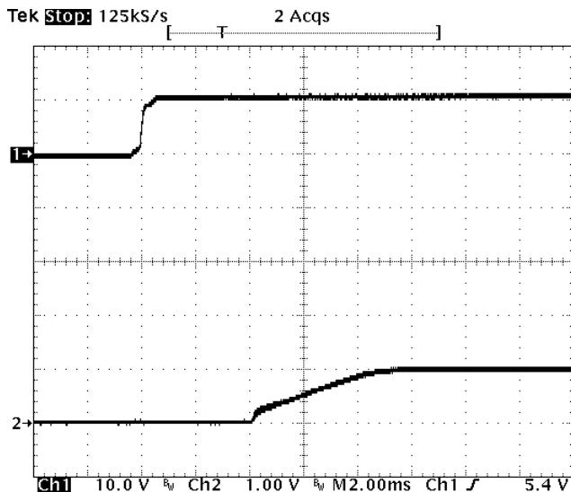
**Fig-1.0V-4:** Turn-on transient for  $V_{out}=1.0V$  with application of  $V_{in}$  at full rated load current (resistive) and  $47\mu F \times 4$  external capacitance at  $V_{in}=12V$ .
