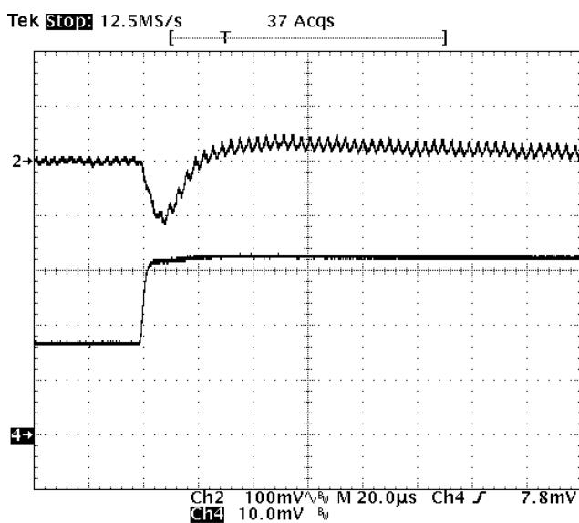
**Fig-2.5V-6:** Output voltage response for  $V_{out}=2.5V$  to positive load current step change from 8A to 16A with slew rate of  $5A/\mu s$  at  $V_{in}=12V$ .  $C_o=47\mu F \times 4$  ceramic.
