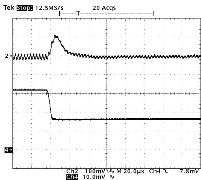
**Fig-3.3V-7:** Output voltage response for  $V_{out}=3.3V$  to negative load current step change from 16A to 8A with slew rate of  $-5A/\mu s$  at  $V_{in}=12V$ .  $C_o=47\mu F \times 4$  ceramic.
