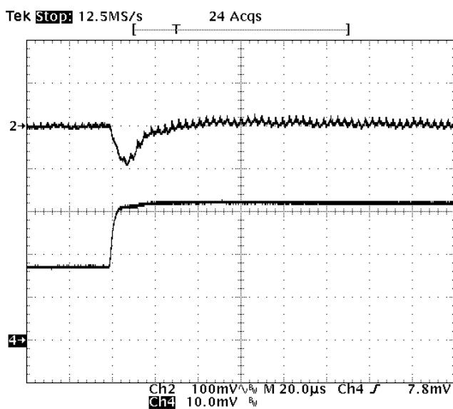
**Fig-1.5V-6:** Output voltage response for  $V_{out}=1.5V$  to positive load current step change from 8A to 16A with slew rate of  $5A/\mu s$  at  $V_{in}=12V$ .  $C_o=47\mu F \times 4$  ceramic.
