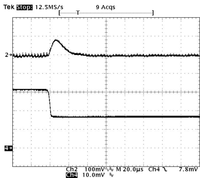
**Fig-1.0V-7:** Output voltage response for  $V_{out}=1.0V$  to negative load current step change from 16A to 8A with slew rate of  $-5A/\mu s$  at  $V_{in}=12V$ .  $C_o=47\mu F \times 4$  ceramic.
