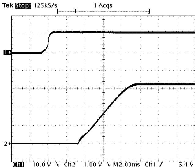
**Fig-3.3V-4:** Turn-on transient for  $V_{out}=3.3V$  with application of  $V_{in}$  at full rated load current (resistive) and  $47\mu F \times 4$  external capacitance at  $V_{in}=12V$ .
