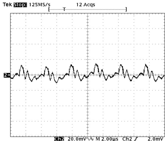
**Fig-1.8V-5:** Output voltage ripple (20mV/div.) for  $V_{out}=1.8V$  at full rated load current into a resistive load with external capacitance  $47\mu F \times 4$  ceramic +  $1\mu F$  ceramic at  $V_{in}=12V$ .
