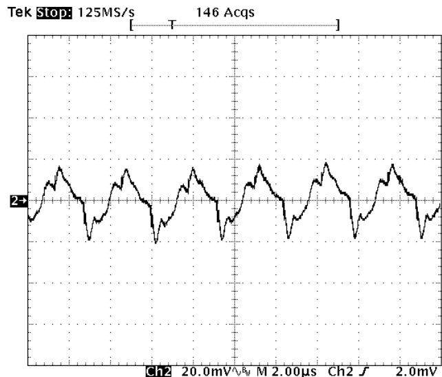
**Fig-5.0V-5:** Output voltage ripple (20mV/div.) for  $V_{out}=5.0V$  at full rated load current into a resistive load with external capacitance  $47\mu F \times 4$  ceramic +  $1\mu F$  ceramic at  $V_{in}=12V$ .
