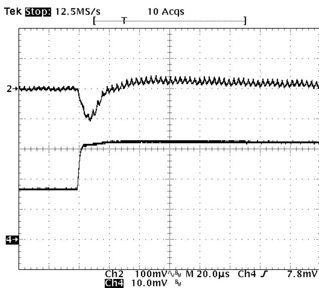
**Fig-2.0V-6:** Output voltage response for  $V_{out}=2.0V$  to positive load current step change from 8A to 16A with slew rate of  $5A/\mu s$  at  $V_{in}=12V$ .  $C_o=47\mu F \times 4$  ceramic.
