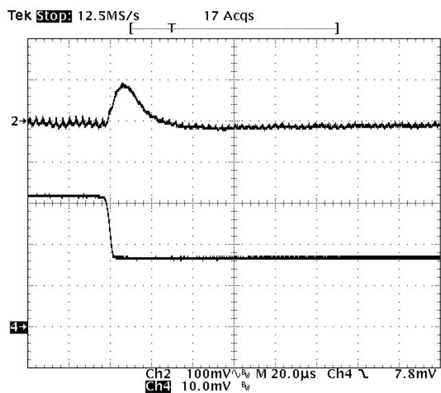
**Fig-1.5V-7:** Output voltage response for  $V_{out}=1.5V$  to negative load current step change from 16A to 8A with slew rate of  $-5A/\mu s$  at  $V_{in}=12V$ .  $C_o=47\mu F \times 4$  ceramic.
