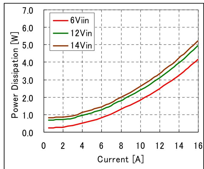
**Fig-3.3V-3:** Power Loss vs. load current and input voltage for  $V_{out}=3.3V$ .
