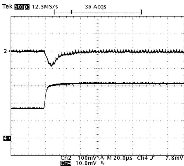
**Fig-1.0V-6:** Output voltage response for  $V_{out}=1.0V$  to positive load current step change from 8A to 16A with slew rate of  $5A/\mu s$  at  $V_{in}=12V$ .  $C_o=47\mu F \times 4$  ceramic.
