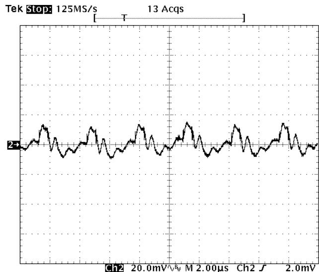
**Fig-2.0V-5:** Output voltage ripple (20mV/div.) for  $V_{out}=2.0V$  at full rated load current into a resistive load with external capacitance  $47\mu F \times 4$  ceramic +  $1\mu F$  ceramic at  $V_{in}=12V$ .
