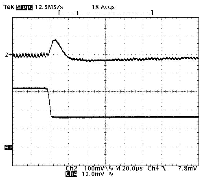
**Fig-2.0V-7:** Output voltage response for  $V_{out}=2.0V$  to negative load current step change from 16A to 8A with slew rate of  $-5A/\mu s$  at  $V_{in}=12V$ .  $C_o=47\mu F \times 4$  ceramic.
