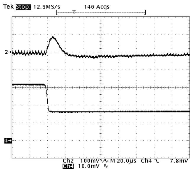
**Fig-1.8V-7:** Output voltage response for  $V_{out}=1.8V$  to negative load current step change from 16A to 8A with slew rate of  $-5A/\mu s$  at  $V_{in}=12V$ .  $C_o=47\mu F \times 4$  ceramic.
