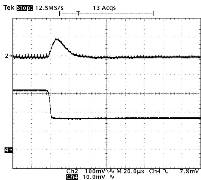
**Fig-1.2V-7:** Output voltage response for  $V_{out}=1.2V$  to negative load current step change from 16A to 8A with slew rate of  $-5A/\mu s$  at  $V_{in}=12V$ .  $C_o=47\mu F \times 4$  ceramic.
