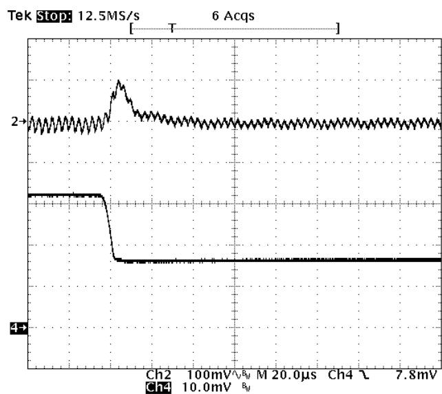
**Fig-5.0V-7:** Output voltage response for  $V_{out}=5.0V$  to negative load current step change from 16A to 8A with slew rate of  $-5A/\mu s$  at  $V_{in}=12V$ .  $C_o=47\mu F \times 4$  ceramic.
