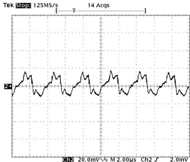
**Fig-3.3V-5:** Output voltage ripple (20mV/div.) for  $V_{out}=3.3V$  at full rated load current into a resistive load with external capacitance  $47\mu F \times 4$  ceramic +  $1\mu F$  ceramic at  $V_{in}=12V$ .
