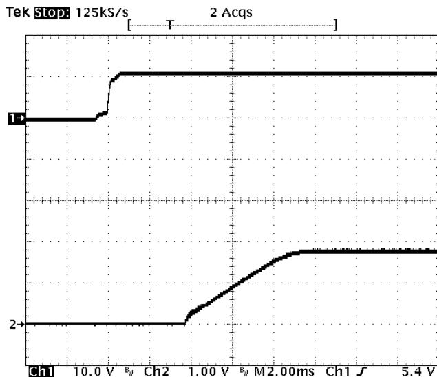
**Fig-1.8V-4:** Turn-on transient for  $V_{out}=1.8V$  with application of  $V_{in}$  at full rated load current (resistive) and  $47\mu F \times 4$  external capacitance at  $V_{in}=12V$ .
