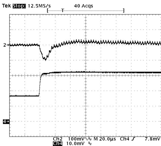
**Fig-1.8V-6:** Output voltage response for  $V_{out}=1.8V$  to positive load current step change from 8A to 16A with slew rate of  $5A/\mu s$  at  $V_{in}=12V$ .  $C_o=47\mu F \times 4$  ceramic.
