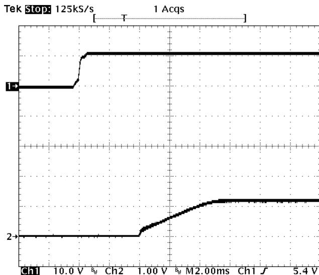
**Fig-1.2V-4:** Turn-on transient for  $V_{out}=1.2V$  with application of  $V_{in}$  at full rated load current (resistive) and  $47\mu F \times 4$  external capacitance at  $V_{in}=12V$ .
