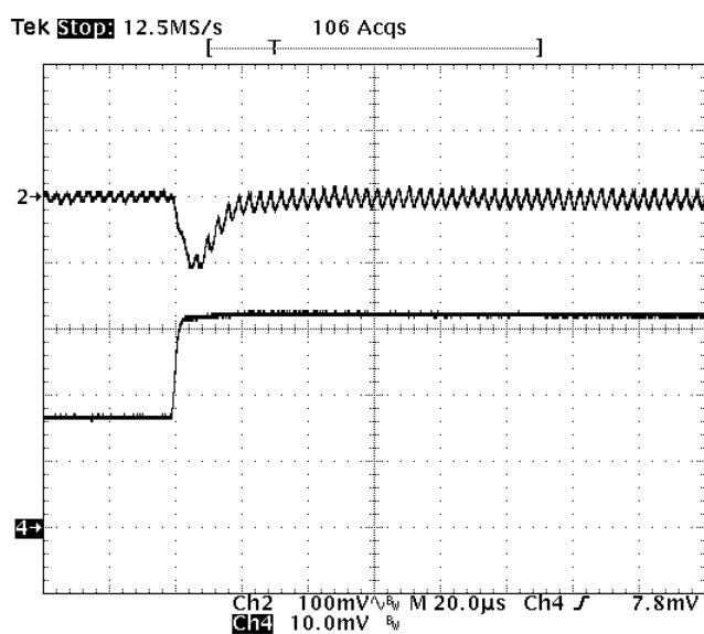
**Fig-3.3V-6:** Output voltage response for  $V_{out}=3.3V$  to positive load current step-change from 8A to 16A with slew rate of  $5A/\mu s$  at  $V_{in}=12V$ .  $C_o=47\mu F \times 4$  ceramic.
