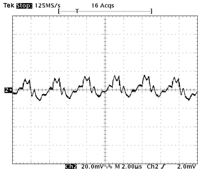
**Fig-2.5V-5:** Output voltage ripple (20mV/div.) for  $V_{out}=2.5V$  at full rated load current into a resistive load with external capacitance  $47\mu F \times 4$  ceramic +  $1\mu F$  ceramic at  $V_{in}=12V$ .
