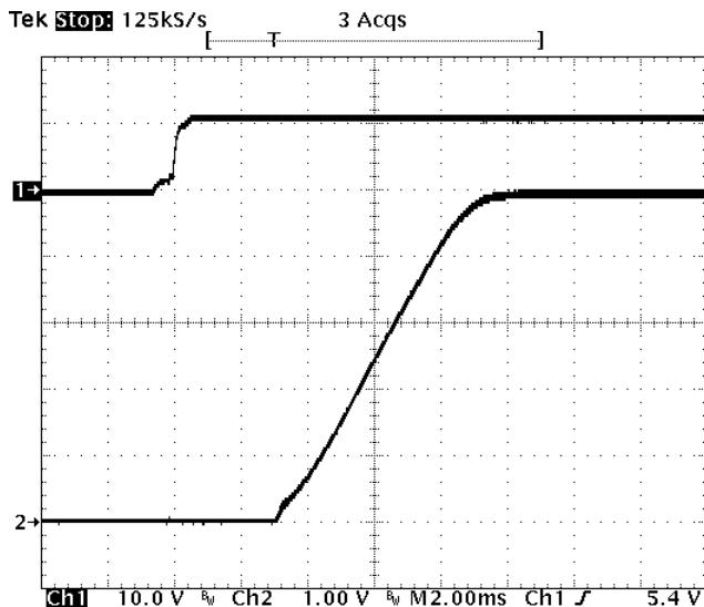
**Fig-5.0V-4:** Turn-on transient for  $V_{out}=5.0V$  with application of  $V_{in}$  at full rated load current (resistive) and  $47\mu F \times 4$  external capacitance at  $V_{in}=12V$ .
