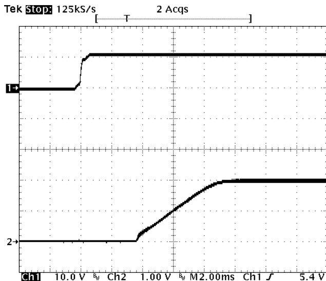
**Fig-2.0V-4:** Turn-on transient for  $V_{out}=2.0V$  with application of  $V_{in}$  at full rated load current (resistive) and  $47\mu F \times 4$  external capacitance at  $V_{in}=12V$ .
