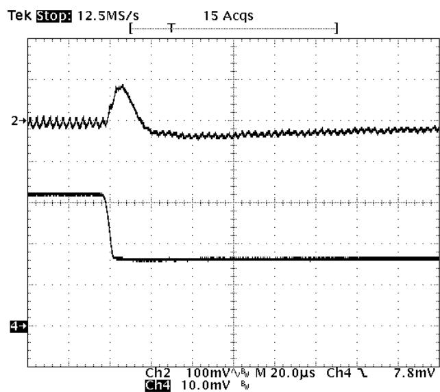
**Fig-2.5V-7:** Output voltage response for  $V_{out}=2.5V$  to negative load current step change from 16A to 8A with slew rate of  $-5A/\mu s$  at  $V_{in}=12V$ .  $C_o=47\mu F \times 4$  ceramic.
