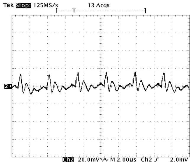
**Fig-1.0V-5:** Output voltage ripple (20mV/div.) for  $V_{out}=1.0V$  at full rated load current into a resistive load with external capacitance  $47\mu F \times 4$  ceramic +  $1\mu F$  ceramic at  $V_{in}=12V$ .
