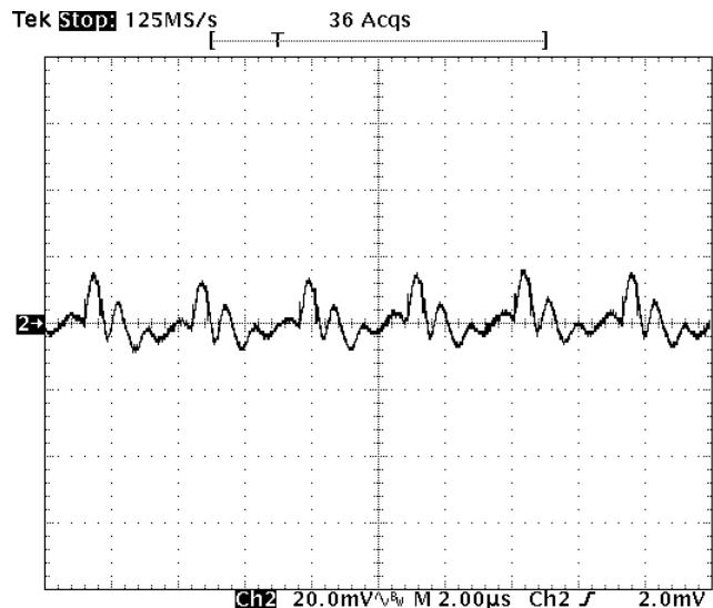
**Fig-1.5V-5:** Output voltage ripple (20mV/div.) for  $V_{out}=1.5V$  at full rated load current into a resistive load with external capacitance  $47\mu F \times 4$  ceramic +  $1\mu F$  ceramic at  $V_{in}=12V$ .
