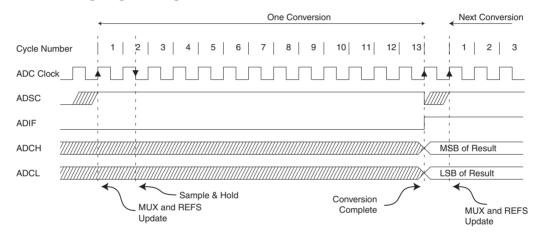
Figure 22-6. ADC Timing Diagram, Auto Triggered Conversion
