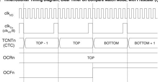
Figure 17-11. Timer/Counter Timing Diagram, Clear Timer on Compare Match Mode, with Prescaler (fclk 1/0/8)
