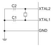
The Oscillator can operate in three different modes, each optimized for a specific frequency range. The operating mode is selected by the fuses CKSEL3:1 as shown in Table 8-3.
