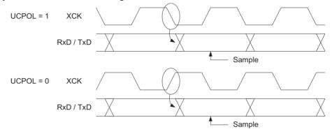
The UCPOL bit UCRSC selects which XCK clock edge is used for data sampling and which is used for data change. As Figure 19-3 shows, when UCPOL is zero the data will be changed at rising XCK edge and sampled at falling XCK edge. If UCPOL is set, the data will be changed at falling XCK edge and sampled at rising XCK edge.
