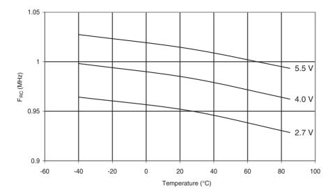
Figure 28-47. Calibrated 1MHz RC Oscillator Frequency vs. V<sub>CC</sub>
