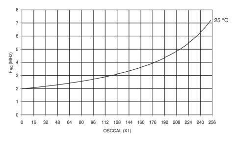
Figure 28-43. Calibrated 2MHz RC Oscillator Frequency vs. Temperature
