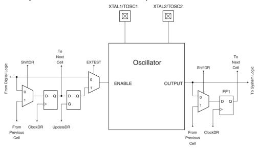
Table 24-3 summaries the scan registers for the external clock pin XTAL1, Oscillators with XTAL1/XTAL2 connections as well as 32 kHz Timer Oscillator.
