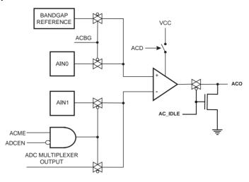
Figure 24-9. General Boundary-scan Cell used for Signals for Comparator and ADC
