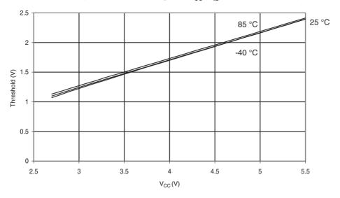
Figure 28-29. I/O Pin Input Hysteresis vs.  $V_{\rm CC}$
