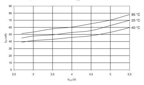
Figure 28-53. Watchdog Timer Current vs.  $V_{\rm CC}$
