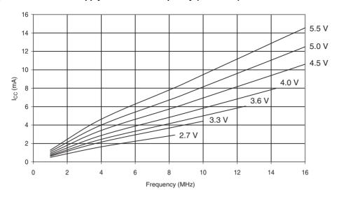
Figure 28-3. Active Supply Current vs. V<sub>CC</sub> (Internal RC Oscillator, 8MHz)
