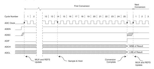
Figure 22-5. ADC Timing Diagram, Single Conversion
