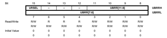
The UBRRH Register shares the same I/O location as the UCSRC Register. See the "Accessing UBRRH/UCSRC Registers" on page 157 section which describes how to access this register.
