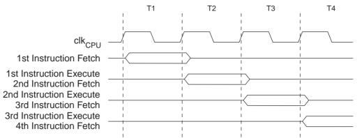
Figure 6-5 shows the internal timing concept for the Register File. In a single clock cycle an ALU operation using two register operands is executed, and the result is stored back to the destination register.
