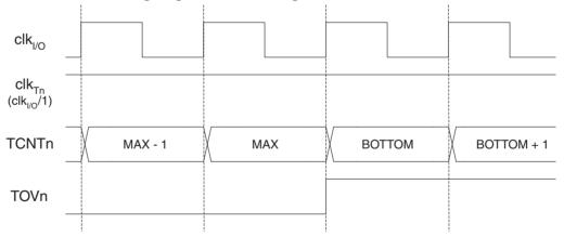
Figure 17-9 shows the same timing data, but with the prescaler enabled.
