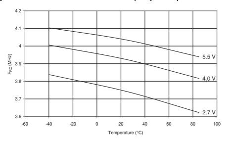
Figure 28-41. Calibrated 4MHz RC Oscillator Frequency vs.  $V_{\rm CC}$
