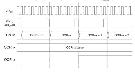
Figure 16-12 shows the count sequence close to TOP in various modes. When using phase and frequency correct PWM mode the OCR1x Register is updated at BOTTOM. The timing diagrams will be the same, but TOP should be replaced by BOTTOM, TOP-1 by BOTTOM+1 and so on. The same renaming applies for modes that set the TOV1 Flag at BOTTOM.
