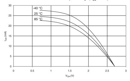
Figure 28-25. I/O Pin Sink Current vs. Output Voltage ( $V_{CC} = 5V$ )
