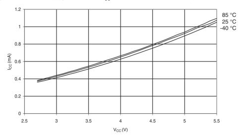
Figure 28-13. Idle Supply Current vs. V<sub>CC</sub> (Internal RC Oscillator, 1MHz)
