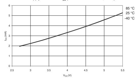
Figure 28-5. Active Supply Current vs. V<sub>CC</sub> (Internal RC Oscillator, 2MHz)
