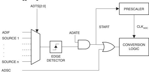
Figure 22-2. ADC Auto Trigger Logic
