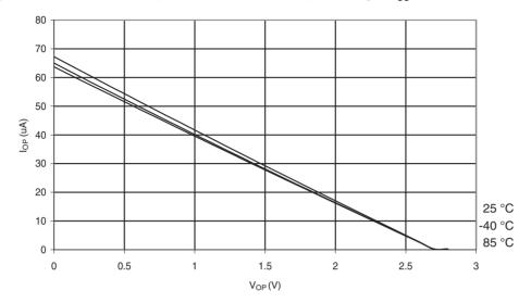
Figure 28-21. Reset Pull-Up Resistor Current vs. Reset Pin Voltage (V<sub>CC</sub> = 5V)
