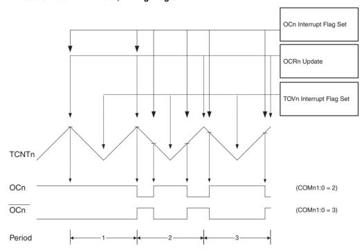
Figure 14-7. Phase Correct PWM Mode, Timing Diagram
