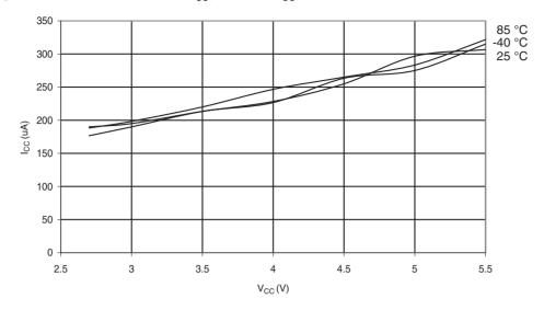
Figure 28-51. Aref External Reference Current vs.  $V_{\rm CC}$
