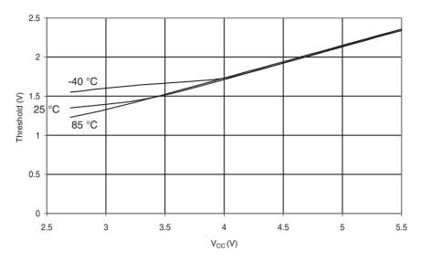
Figure 28-31. Reset Input Threshold Voltage vs. V<sub>CC</sub> (V<sub>IL</sub>, Reset Pin Read As '0')
