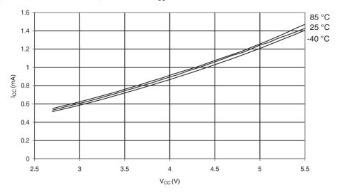
Figure 28-7. Active Supply Current vs. V<sub>CC</sub> (32kHz External Oscillator)
