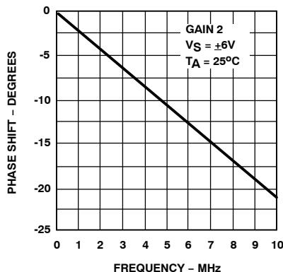
**Figure 20.** Phase Shift as a Function of Frequency
