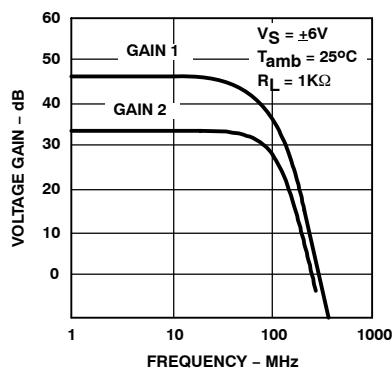
**Figure 22.** Voltage Gain as a Function of Frequency
