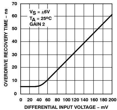
Figure 15. Differential Overdrive Recovery Time
