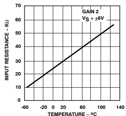
Figure 18. Input Resistance as a Function of Temperature
