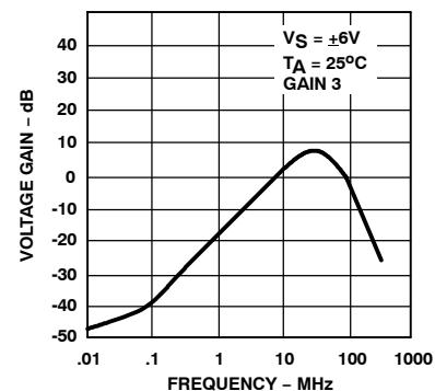
**Figure 23.** Voltage Gain as a Function of Frequency
