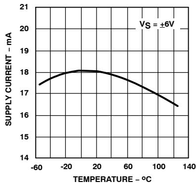
Figure 14. Supply Current as a Function of Temperature
