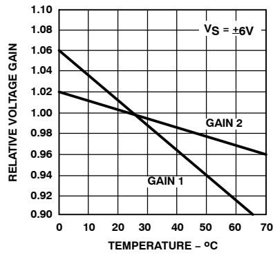
Figure 8. Voltage Gain as a Function of Temperature
