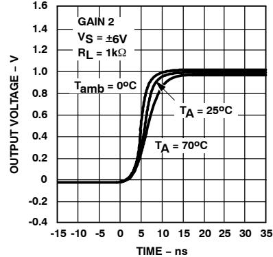
Figure 7. Pulse Response as a Function of Temperature
