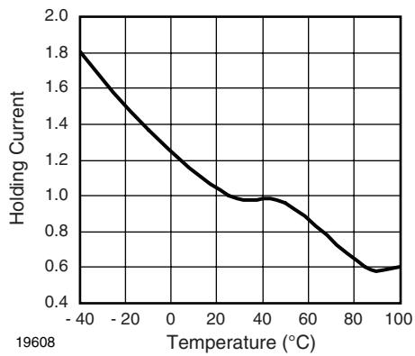
Fig. 7 - Normalized Holding Current vs. Temperature
