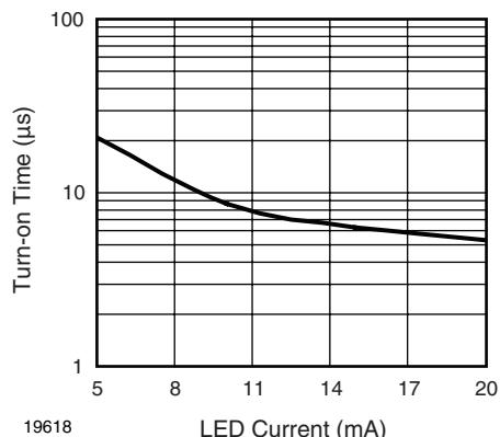
Fig. 6 - Turn-on Time vs. LED Current
