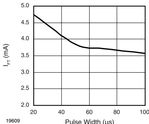
Fig. 9 - Trigger Current vs. Pulse Width
