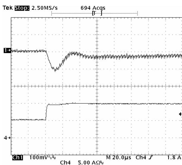
**Fig-1.0V-6:** Output voltage response for  $V_{out}=1.0V$  to positive load current step-change from  $5A$  to  $10A$  with slew rate of  $5A/\mu s$  at  $V_{in}=5.0V$ .  $C_o=47\mu F \times 4$  ceramic +  $1\mu F$  ceramic.
