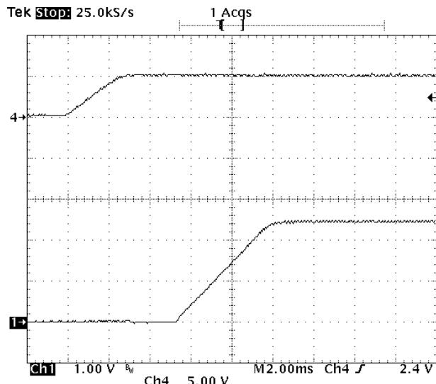
**Fig-2.5V-4:** Turn-on transient for  $V_{out}=2.5V$  with application of  $V_{in}$  at full rated load current (resistive) and  $47\mu F \times 4$  external capacitance at  $V_{in}=5.0V$ .
