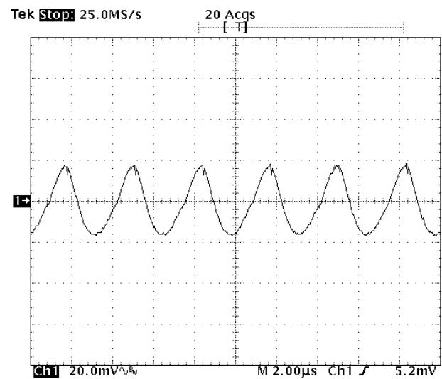
**Fig-1.0V-5:** Output voltage ripple (20mV/div.) for  $V_{out}=1.0V$  at full rated load current into a resistive load with external capacitance  $47\mu F \times 4$  ceramic +  $1\mu F$  ceramic at  $V_{in}=5.0V$ .
