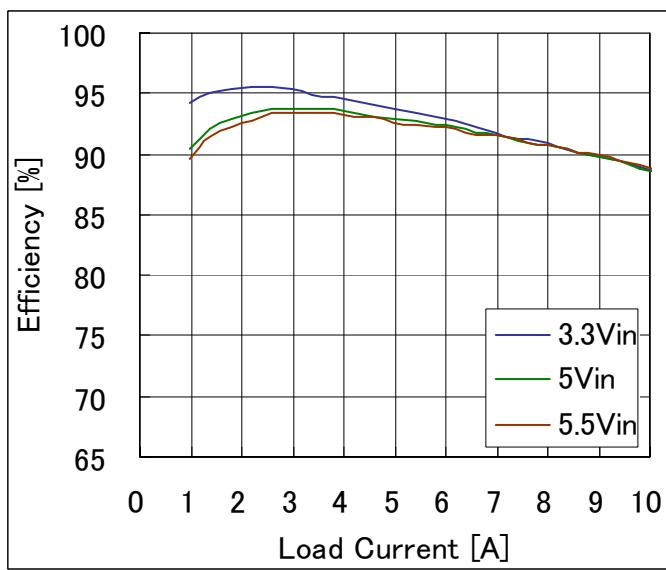
**Fig-2.5V-2:** Efficiency vs. load current and input voltage for  $V_{out}=2.5V$ .
