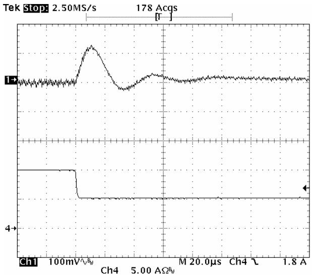
**Fig-1.8V-7:** Output voltage response for  $V_{out}=1.8V$  to positive load current step-change from 10A to 5A with slew rate of  $-5A/\mu s$  at  $V_{in}=5.0V$ .  $C_o=47\mu F \times 4$  ceramic +  $1\mu F$  ceramic.
