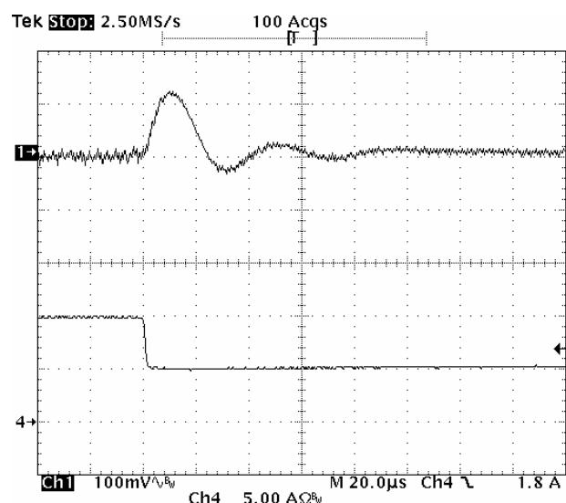
**Fig-2.0V-7:** Output voltage response for  $V_{out}=2.0V$  to positive load current step-change from  $10A$  to  $5A$  with slew rate of  $-5A/\mu s$  at  $V_{in}=5.0V$ .  $C_o=47\mu F \times 4$  ceramic +  $1\mu F$  ceramic.
