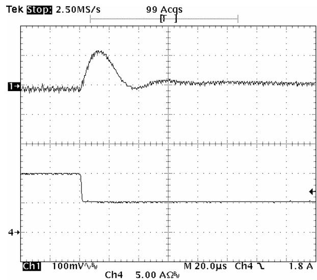
**Fig-1.2V-7:** Output voltage response for  $V_{out}=1.2V$  to positive load current step-change from 10A to 5A with slew rate of  $-5A/\mu s$  at  $V_{in}=5.0V$ .  $C_o=47\mu F \times 4$  ceramic +  $1\mu F$  ceramic.
