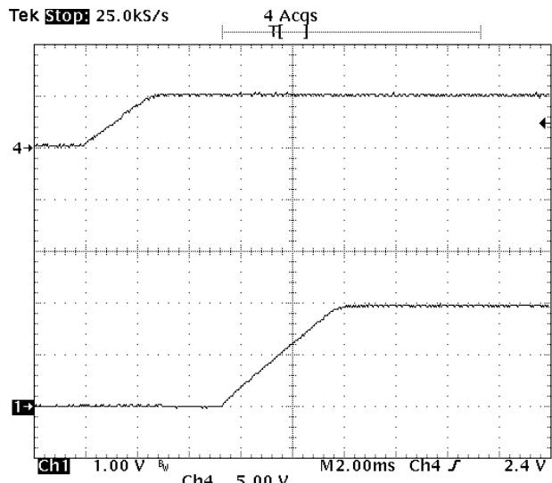
**Fig-2.0V-4:** Turn-on transient for  $V_{out}=2.0V$  with application of  $V_{in}$  at full rated load current (resistive) and  $47\mu F \times 4$  external capacitance at  $V_{in}=5.0V$ .
