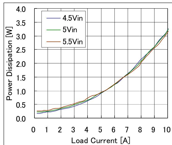
**Fig-3.3V-3:** Power dissipation vs. load current and input voltage for  $V_{out}=3.3V$ . Airflow rate=200 LFM (1.0m/s) and  $T_a=25^{\circ}C$ .
