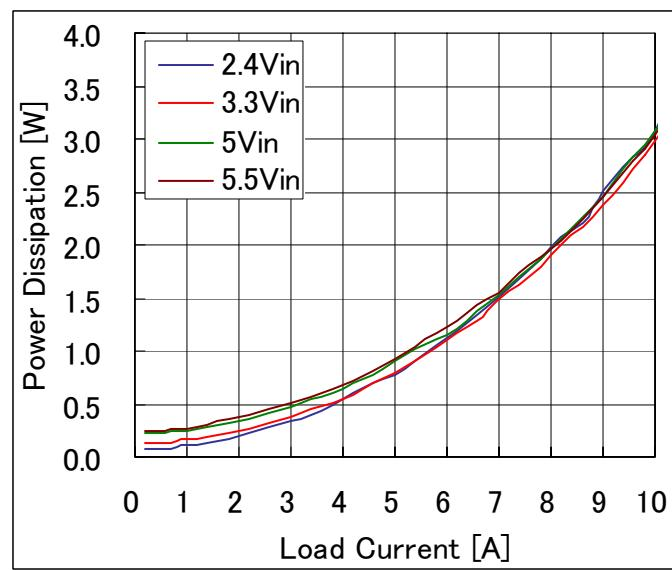
**Fig-1.8V-3:** Power dissipation vs. load current and input voltage for  $V_{out}=1.8V$ . Airflow rate=200 LFM (1.0m/s) and  $T_a=25^{\circ}C$ .
