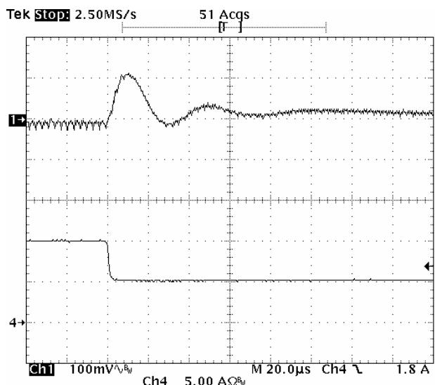
**Fig-2.5V-7:** Output voltage response for  $V_{out}=2.5V$  to positive load current step-change from 10A to 5A with slew rate of  $-5A/\mu s$  at  $V_{in}=5.0V$ .  $C_o=47\mu F \times 4$  ceramic +  $1\mu F$  ceramic.
