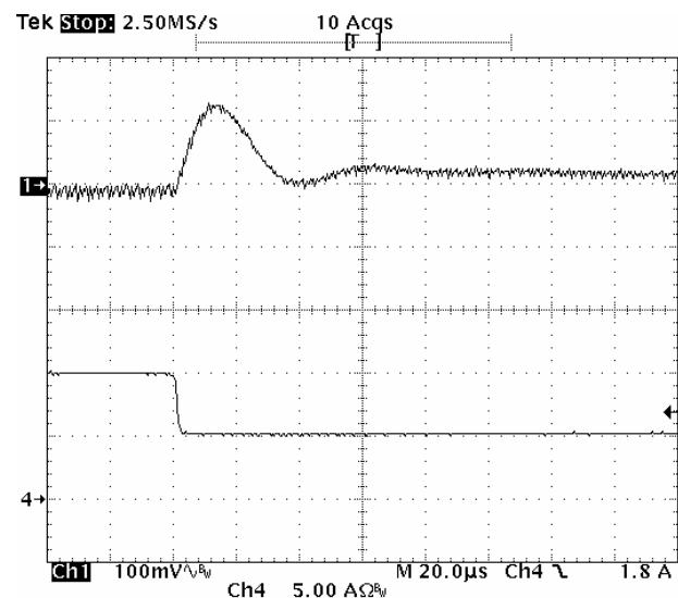
**Fig-1.0V-7:** Output voltage response for  $V_{out}=1.0V$  to positive load current step-change from  $10A$  to  $5A$  with slew rate of  $-5A/\mu s$  at  $V_{in}=5.0V$ .  $C_o=47\mu F \times 4$  ceramic +  $1\mu F$  ceramic.
