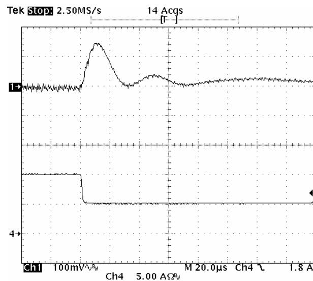
**Fig-3.3V-7:** Output voltage response for  $V_{out}=3.3V$  to positive load current step-change from 10A to 5A with slew rate of  $-5A/\mu s$  at  $V_{in}=5.0V$ .  $C_o=47\mu F \times 4$  ceramic +  $1\mu F$  ceramic.
