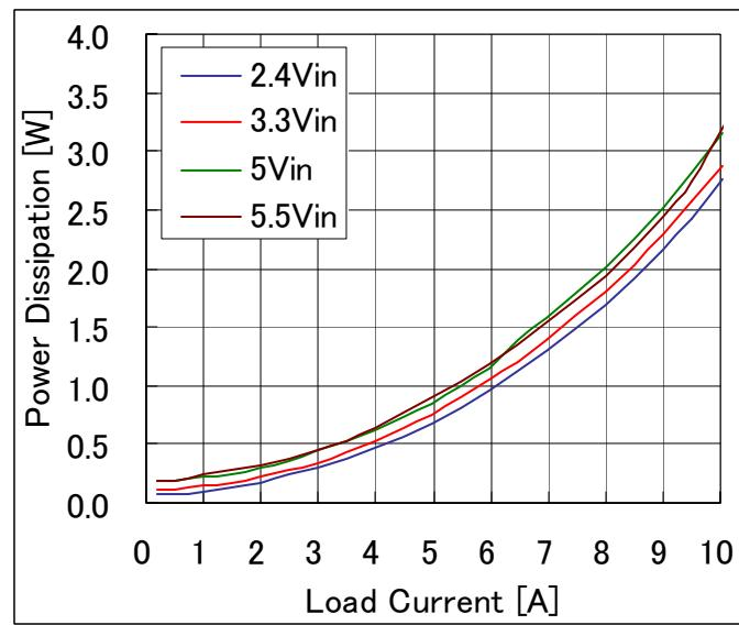
**Fig-0.7525V-3:** Power dissipation vs. load current and input voltage for  $V_{out}=0.7525V$ . Airflow rate=200 LFM (1.0m/s) and  $T_a=25^{\circ}C$ .
