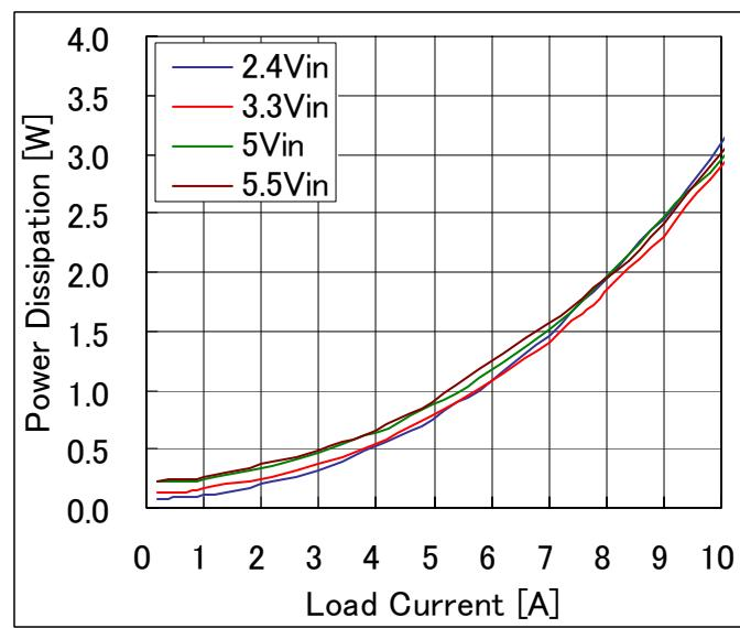
**Fig-1.5V-3:** Power dissipation vs. load current and input voltage for  $V_{out}=1.5V$ . Airflow rate=200 LFM (1.0m/s) and  $T_a=25^{\circ}C$ .
