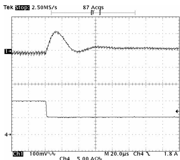
**Fig-0.7525V-7:** Output voltage response for  $V_{out}=0.7525V$  to positive load current step-change from  $10A$  to  $5A$  with slew rate of  $-5A/\mu s$  at  $V_{in}=5.0V$ .  $C_o=47\mu F \times 4$  ceramic +  $1\mu F$  ceramic.
