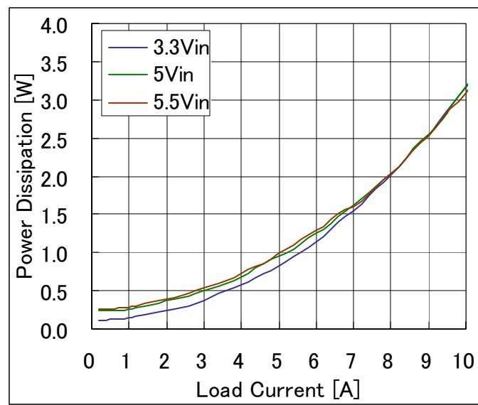
**Fig-2.5V-3:** Power dissipation vs. load current and input voltage for  $V_{out}=2.5V$ .
