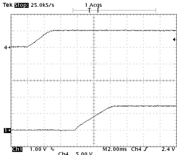
**Fig-1.5V-4:** Turn-on transient for  $V_{out}=1.5V$  with application of  $V_{in}$  at full rated load current (resistive) and  $47\mu F \times 4$  external capacitance at  $V_{in}=5.0V$ .
