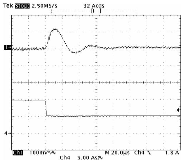
**Fig-1.5V-7:** Output voltage response for  $V_{out}=1.5V$  to positive load current step-change from 10A to 5A with slew rate of  $-5A/\mu s$  at  $V_{in}=5.0V$ .  $C_o=47\mu F \times 4$  ceramic +  $1\mu F$  ceramic.
