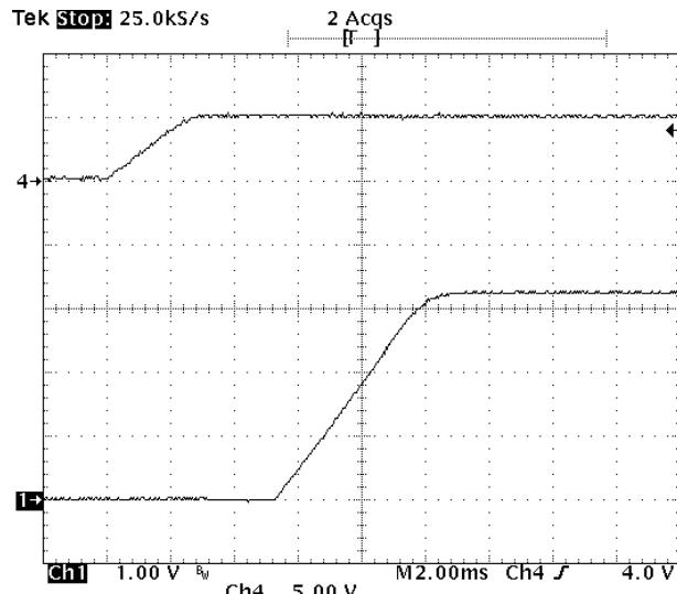
**Fig-3.3V-4:** Turn-on transient for  $V_{out}=3.3V$  with application of  $V_{in}$  at full rated load current (resistive) and  $47\mu F \times 4$  external capacitance at  $V_{in}=5.0V$ .
