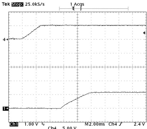
**Fig-1.2V-4:** Turn-on transient for  $V_{out}=1.2V$  with application of  $V_{in}$  at full rated load current (resistive) and  $47\mu F \times 4$  external capacitance at  $V_{in}=5.0V$ .
