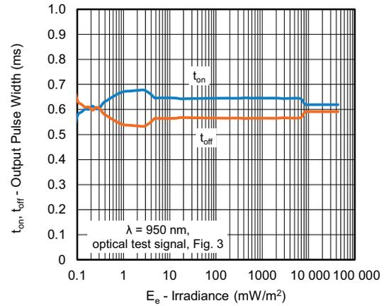
Fig. 4 - Pulse-Width vs. Irradiance in Dark Ambient
