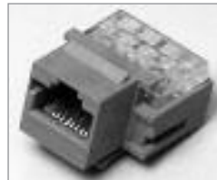
90° Cat3 Tool-less Keystone USOC Jacks (Voice - 6p6c)
