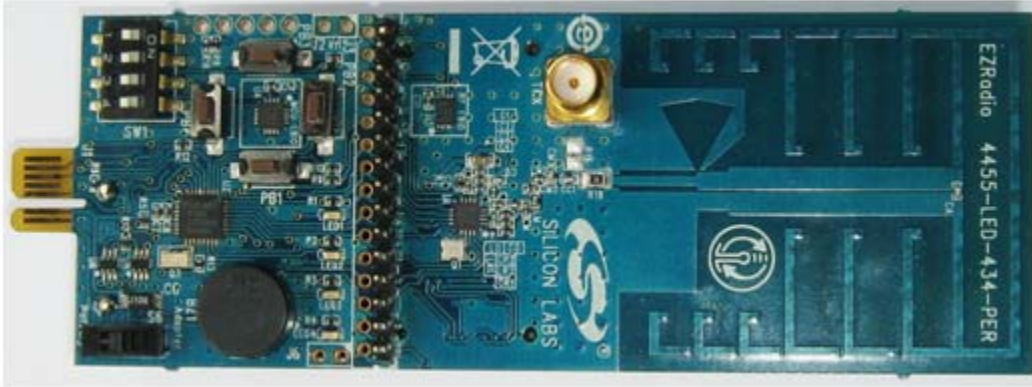
Figure 1. Si4455 RFStick 434 MHz Transceiver Board (P/N 4455-LED-434-PER)
