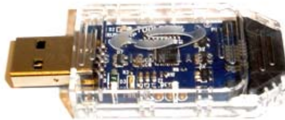
Figure 2. Toolstick Base Adapter (P/N Toolstick_BA)
