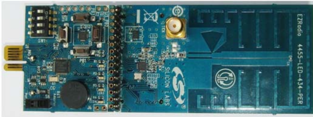
Figure 1. Si4455 RFStick 434 MHz Transceiver Board (P/N 4455-LED-434-PER)
