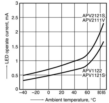
4. LED turn off current vs. ambient temperature characteristics
