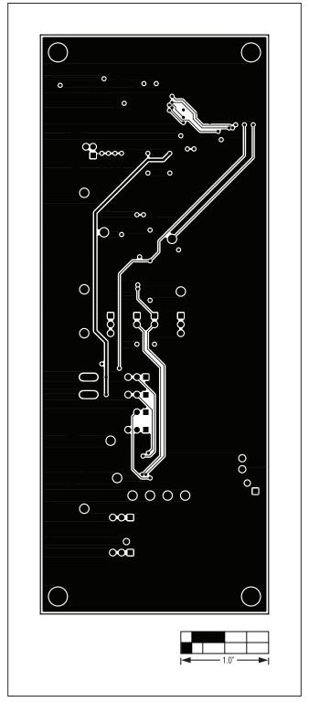
Figure 9. MAX14578 EV Kit PCB Layout—Solder Side
