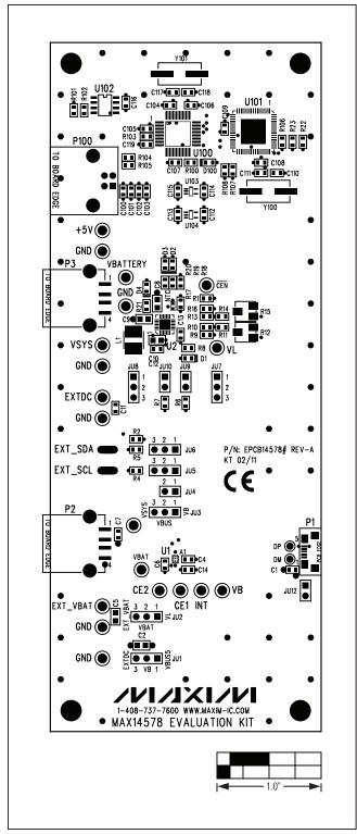
Figure 5. MAX14578 EV Kit Component Placement Guide— Component Side
