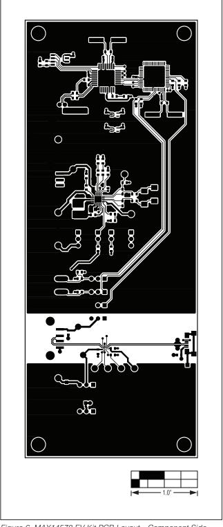
Figure 6. MAX14578 EV Kit PCB Layout—Component Side
