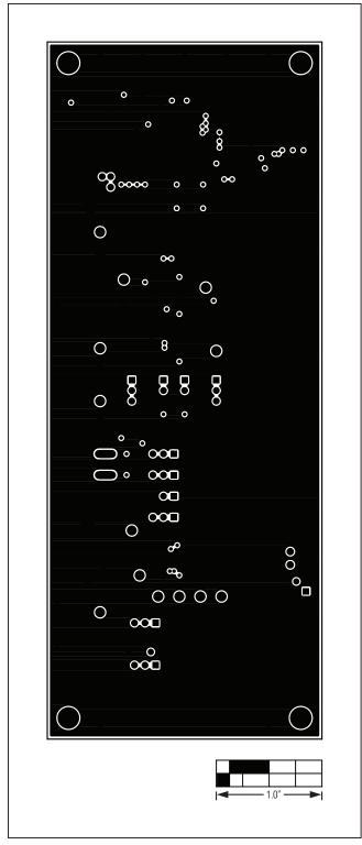
Figure 7. MAX14578 EV Kit PCB Layout—Layer 2
