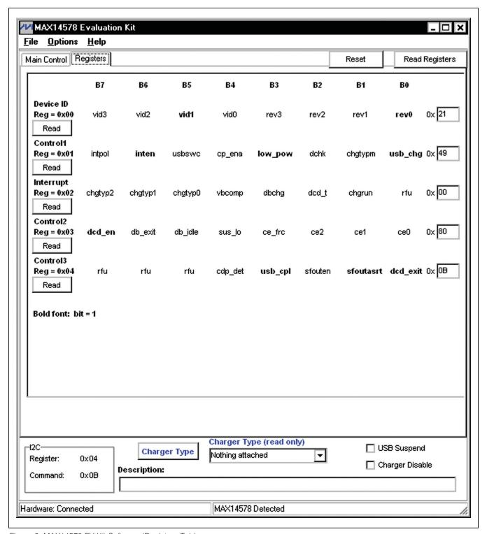
Figure 2. MAX14578 EV Kit Software (Registers Tab)
