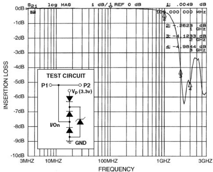
Figure 1. Insertion Loss (S<sub>21</sub>) vs. Frequency (0 V DC Bias, V<sub>p</sub>=3.3 V, MSOP-10 Package)
