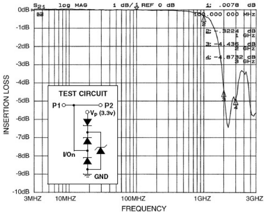
Figure 2. Insertion Loss (S<sub>21</sub>) vs. Frequency (2.5 V DC Bias, V<sub>p</sub>=3.3 V, MSOP-10 Package)
