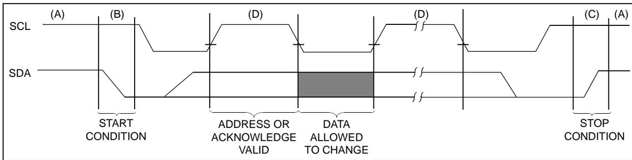
FIGURE 5-7: Data Transfer Sequence on I<sup>2</sup>C Serial Bus.
