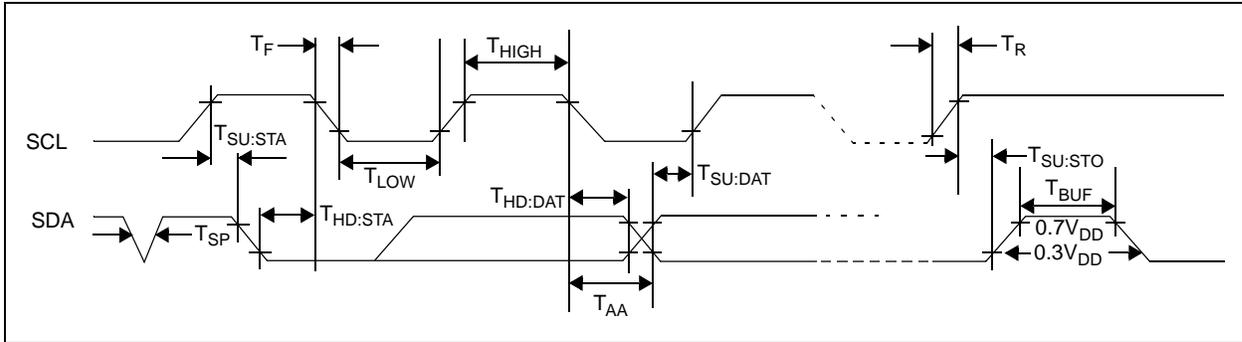
**FIGURE 5-8:** I<sup>2</sup>C Bus Timing Data.
