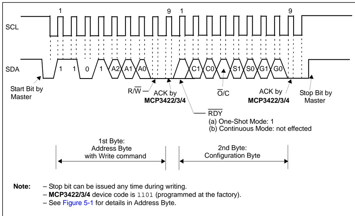
**FIGURE 5-3: Timing Diagram For Writing To The MCP3422/3/4.**
