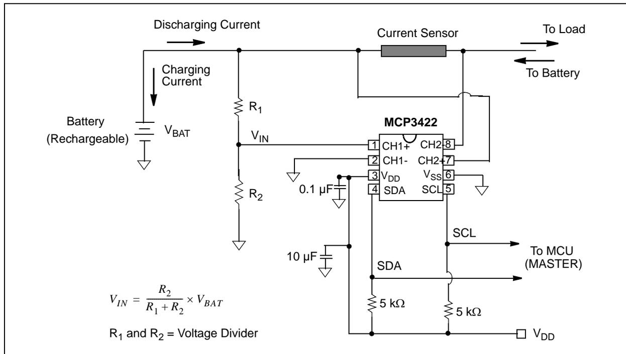
**FIGURE 6-5:** Battery Voltage and Charging/Discharging Current Measurement.
