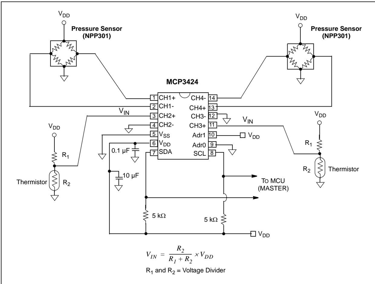
**FIGURE 6-7:** Example of Pressure and Temperature Measurement.
