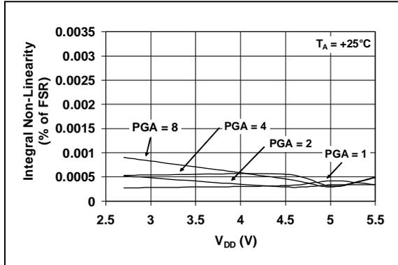
**FIGURE 2-1:** INL vs. Supply Voltage ( $V_{DD}$ ).
