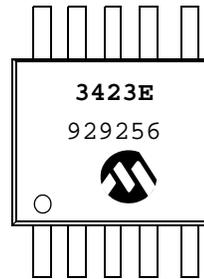
14-Lead SOIC (150 mil) (MCP3424)
