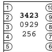
10-Lead MSOP (MCP3423)
