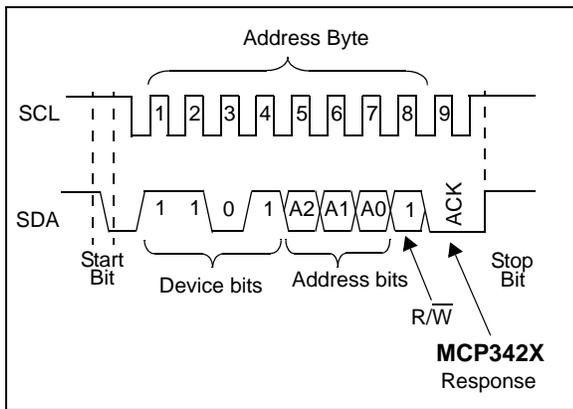
**FIGURE 6-3:** I<sup>2</sup>C Bus Connection Test.
