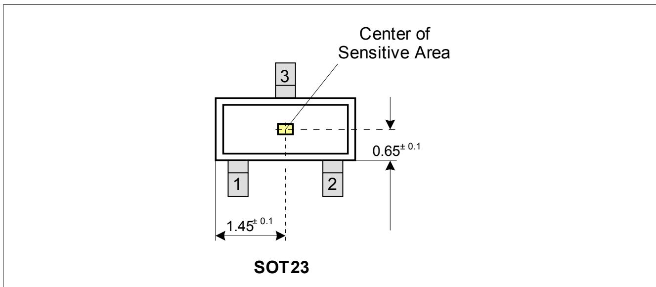
Figure 2 Pin Configuration and Center of Sensitive Area
