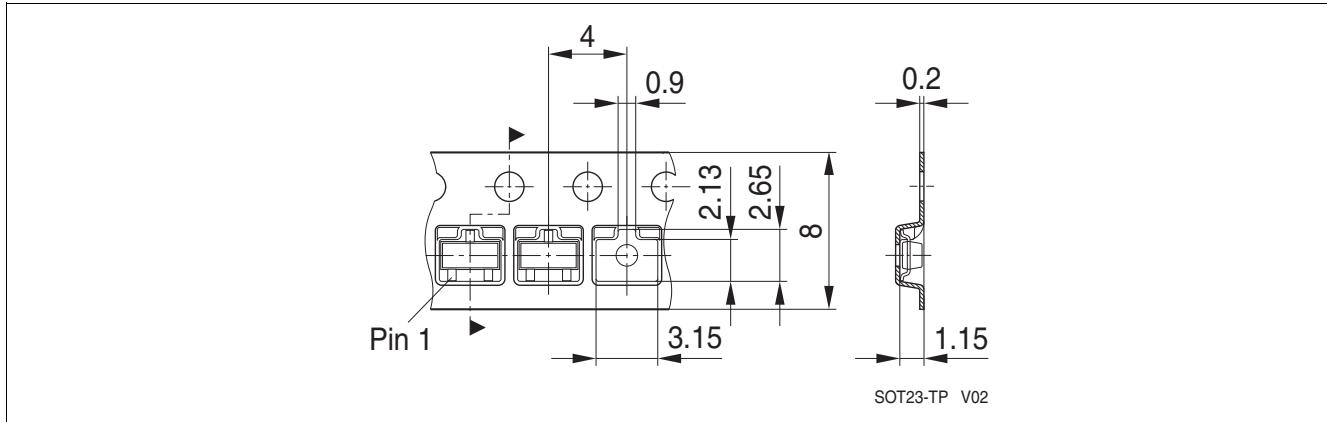
Figure 11 Packing of the PG-SOT23-3-15 in a Tape
