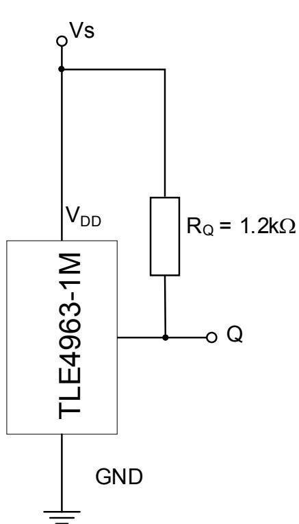
**Figure 7 Application Circuit**
