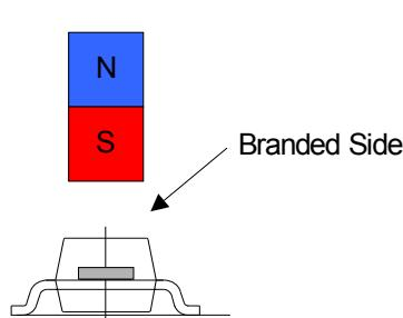
**Figure 8 Definition of Magnetic Field Direction PG-SOT23-3-15**
