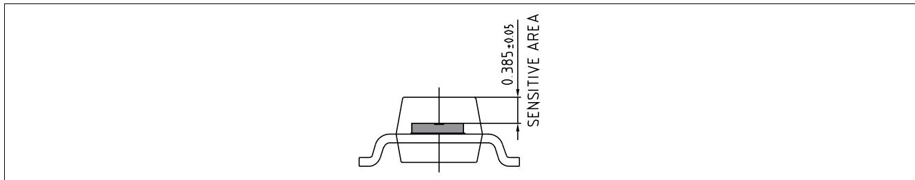
Figure 12 Distance between Chip and Package
