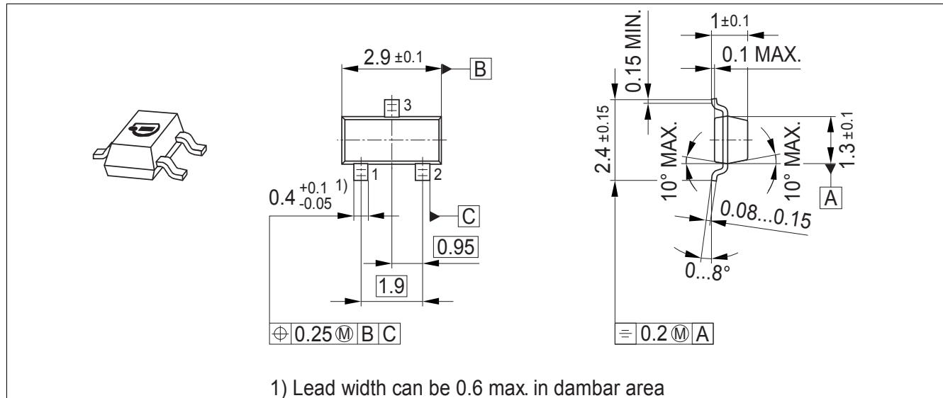
**Figure 9** PG-SOT23-3-15 Package Outline (All Dimensions in mm)
