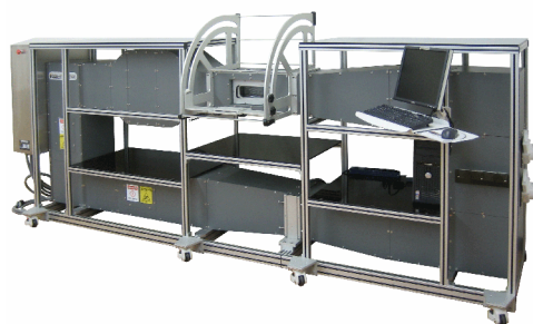
FDK Original Wind Tunnel
