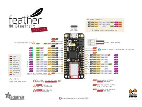
Note AREF in the diagram should be marked PA03 not PA02
