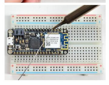
Add the breakout board: Place the breakout board over the pins so that the short pins poke through the breakout pads
