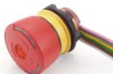
Emergency-stop red LED illuminated, ribbon cable, twist release, 32mm diameter for 22.5mm mounting, foolproof to EN 60947-5-5, EN418
