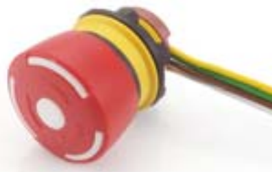
Emergency-stop non illuminated, ribbon cable, twist release, 32mm diameter for 22.5mm mounting, foolproof to EN 60947-5-5, EN 418
