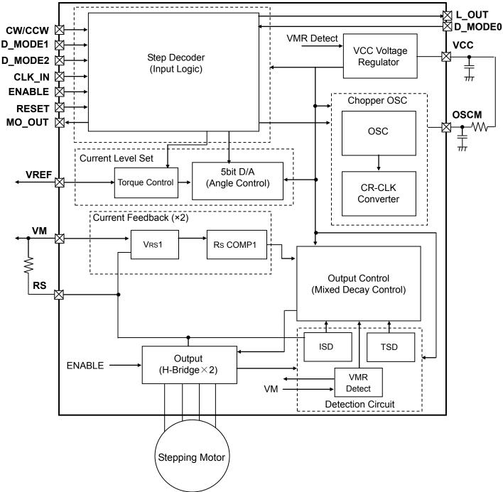
Functional blocks/circuits/constants in the block chart etc. may be omitted or simplified for explanatory purposes.
