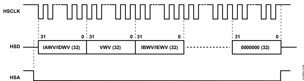
Figure 48. HSDC Communication for HGAP = 0, HXFER[1:0] = 01, and HSAPOL = 0; HSIZE Is Irrelevant
