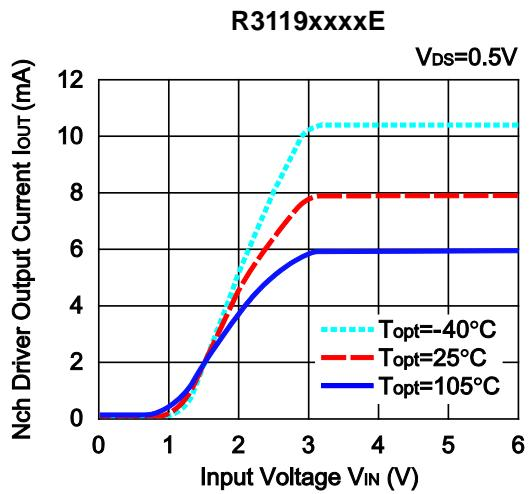
**13) Nch Driver Output Current vs.  $V_{DS}$**
