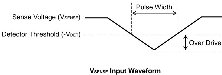
This graph shows the maximum pulse conditions to keep the released voltage. If the pulse with larger amplitude or wider width than the graph above, is input to the V<sub>DD</sub> pin (R3119xxxxA) or to the SENSE pin (R3119xxxxE), the reset signal may be output.
