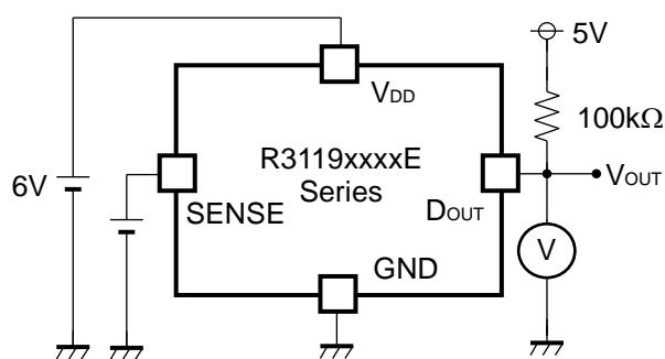
Detector Threshold Test Circuit
