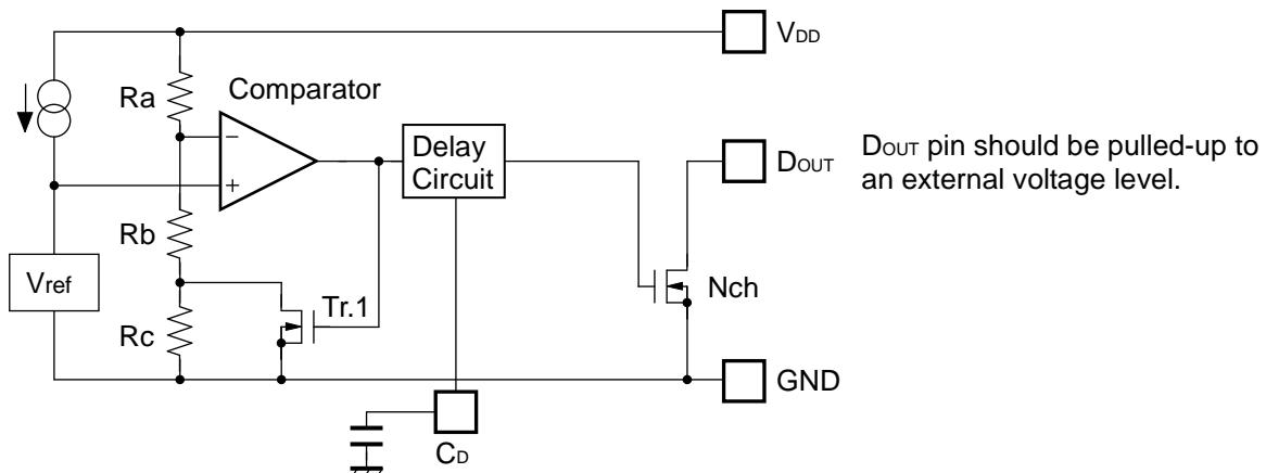
Block Diagram of External Capacitor Connection
