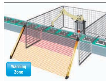
A single sensor zone can also be divided
