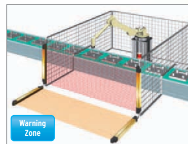
Dividing the zone between series-connected sensors
