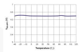
Figure 6. V<sub>DD-OFF1</sub> vs. Temperature
