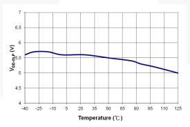
Figure 9. V<sub>DD-OLP</sub> vs. Temperature
