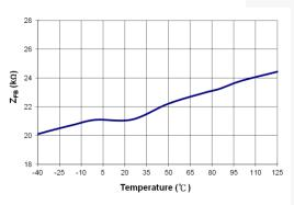
Figure 15. Z<sub>FB</sub> vs. Temperature
