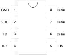
Figure 4. Pin Assignment
