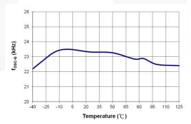
Figure 18. f<sub>OSC-G</sub> vs. Temperature
