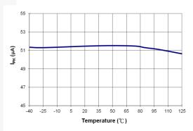
Figure 16. I<sub>PK</sub> vs. Temperature
