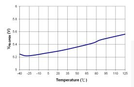
Figure 13. V<sub>FB-OPEN</sub> vs. Temperature
