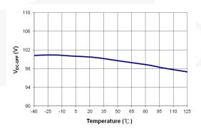
Figure 12.  $V_{\text{DC-OFF}}$  vs. Temperature
