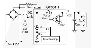
Figure 19. Startup Circuit
