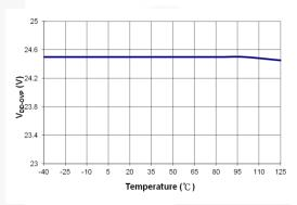
Figure 8. V<sub>DD-OVP</sub> vs. Temperature
