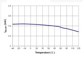
Figure 10. I<sub>DD-OP1</sub> vs. Temperature
