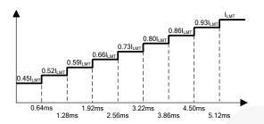
Figure 22. Current Limit Variation During Soft-Start
