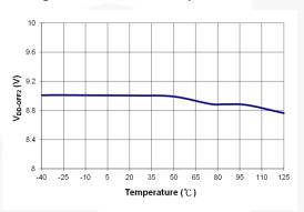
Figure 7. V<sub>DD-OFF2</sub> vs. Temperature
