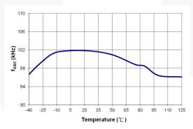
Figure 17. fosc vs. Temperature
