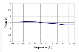
Figure 14. V<sub>FB-OLP</sub> vs. Temperature
