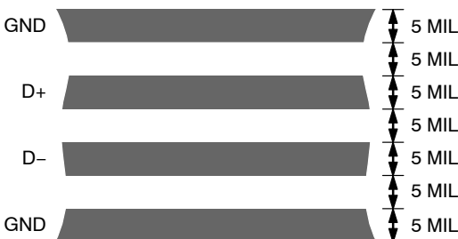
Figure 21. Typical Arrangement of Signal Tracks
