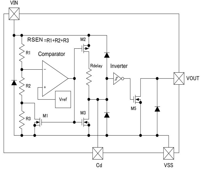
\* Diodes inside the circuits are ESD protection diodes and parasitic diodes.
