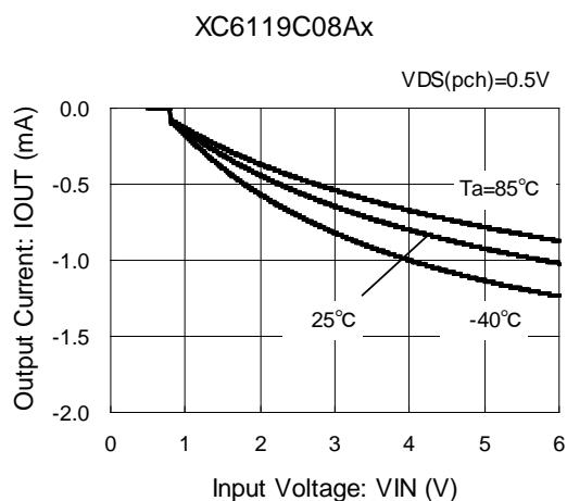
(6) Cd Pin Sink Current vs. Input Voltage
